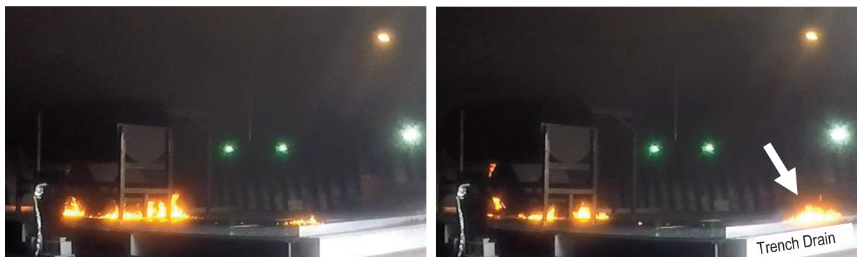
Figure 16. Re-ignition of Fuel vapors on the ILDFA
