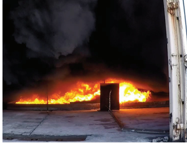
Figure 29. Fire Vortex Adjacent to the South Perimeter Heat Flux Sensor
