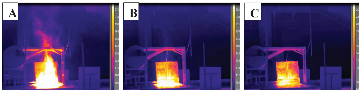
Figure 15. Infrared Images of a 30 gal ILDFA Fuel Spill Fire at 15 s (A), 90 s (B), and 180 s (C) Time Points
