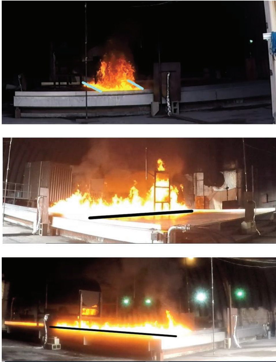
Figure 12. Oval Shape of fire on ILDFA floor
