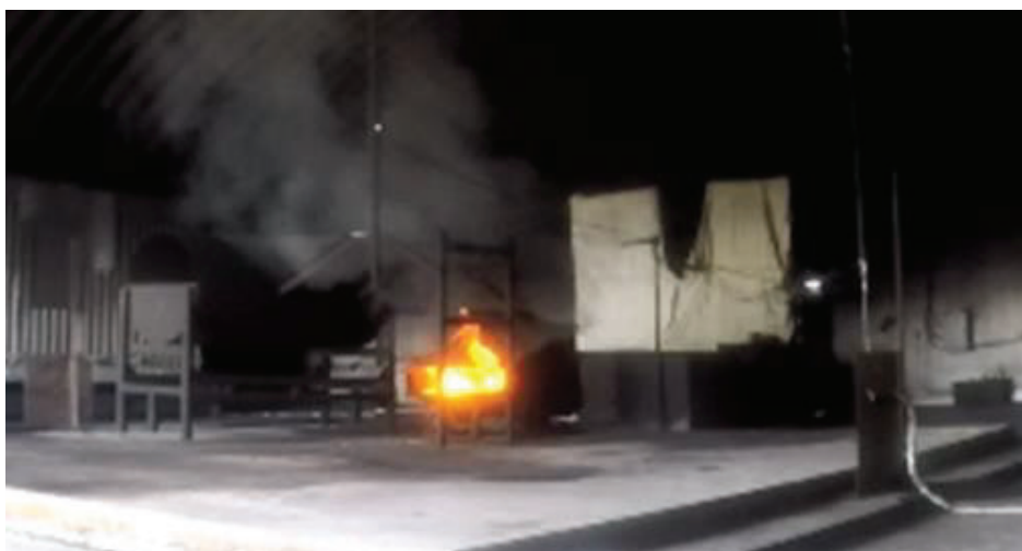
Figure 9. Fuel “Pre-burn” Before Fuel Spill on Concrete
