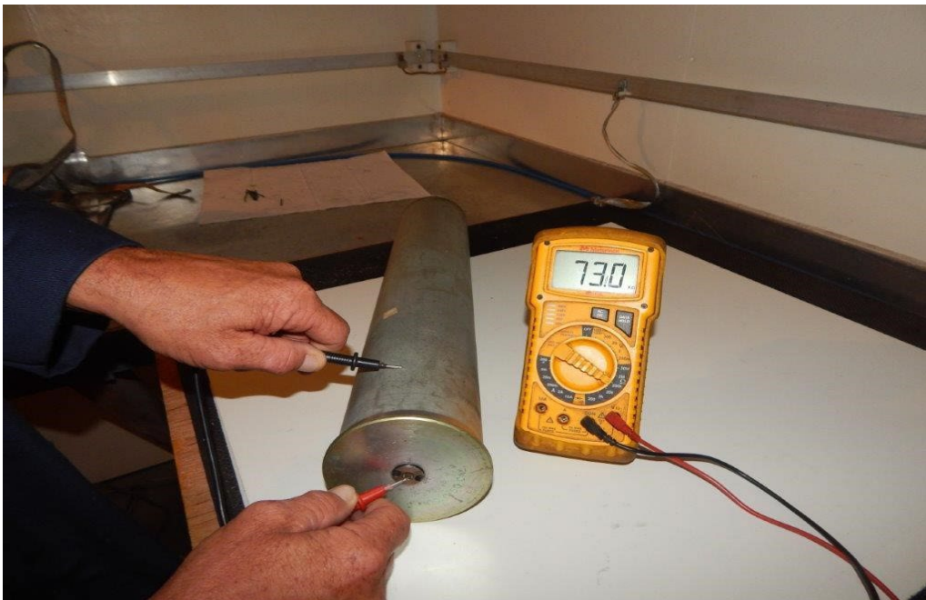
Fig. 20 Resistance check on the primer through the case
