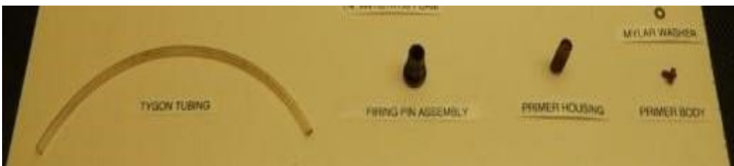
Fig. 2 A firing pin/housing assembly with a 6-inch piece of 1/8-inch ID Tygon tubing and a Mylar washer
