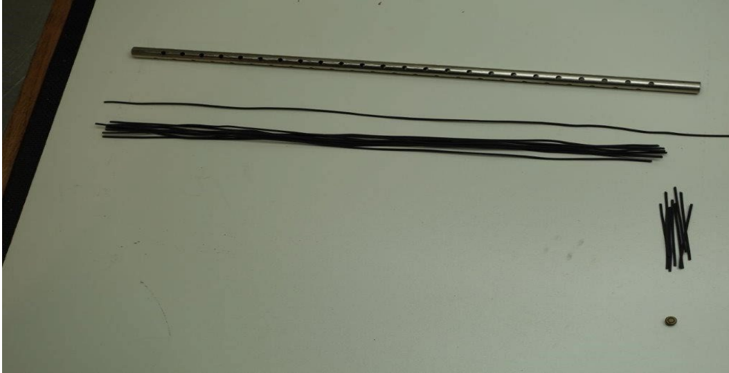
Fig. 8 Trimmed pieces of Benite propellant strands and one strand untrimmed
