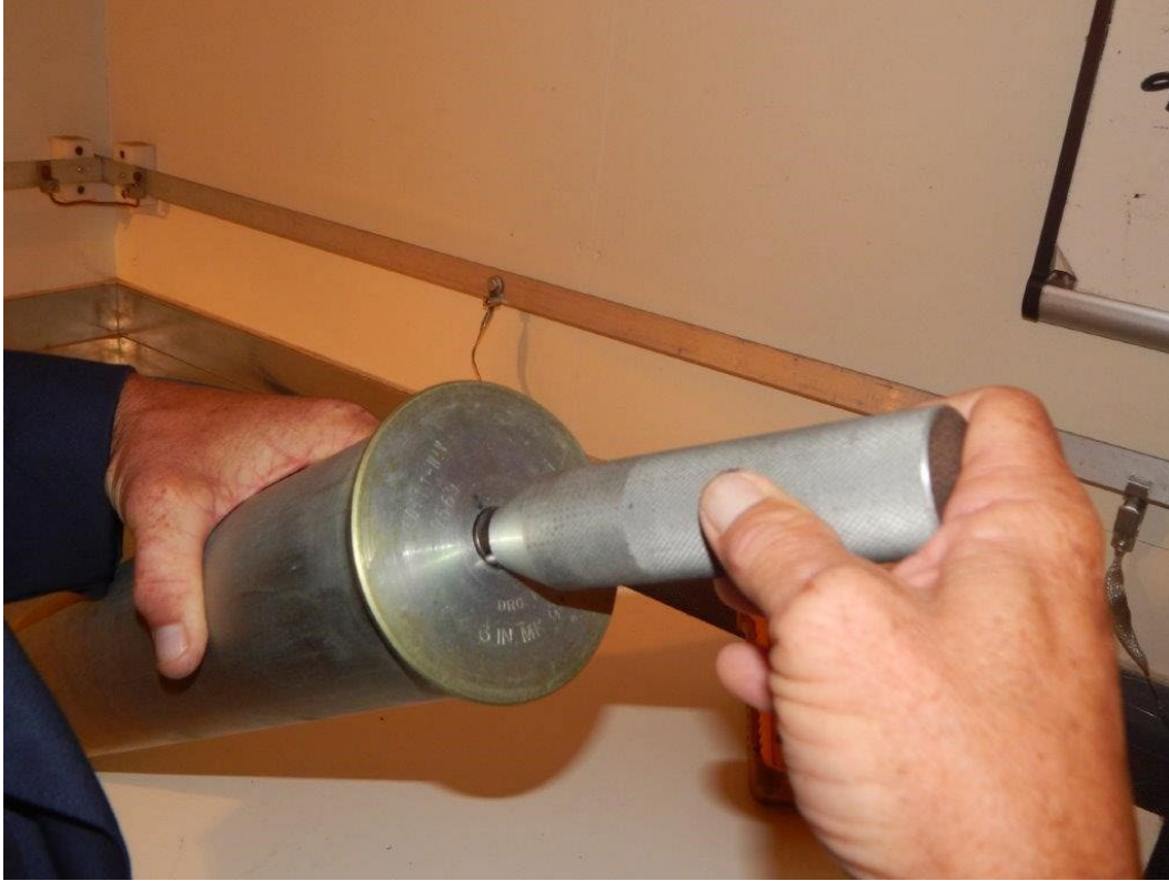
Fig. 14 Primer and spit tube assembly threaded into the case
