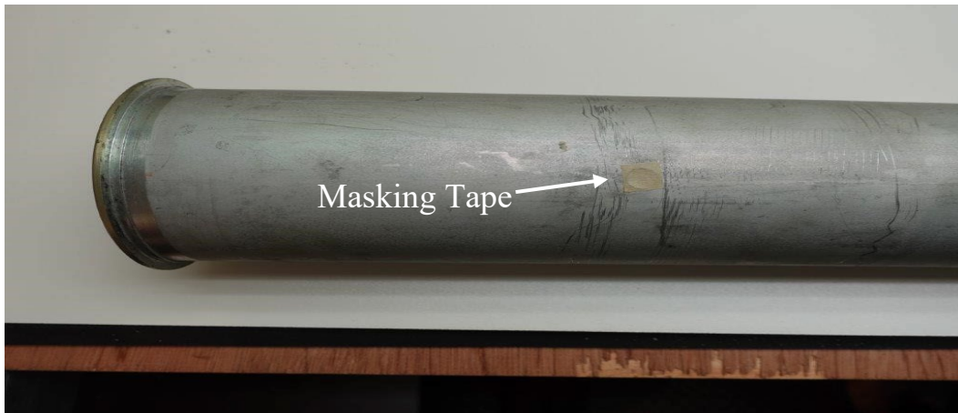
Fig. 5 Tape covering the pressure port hole
