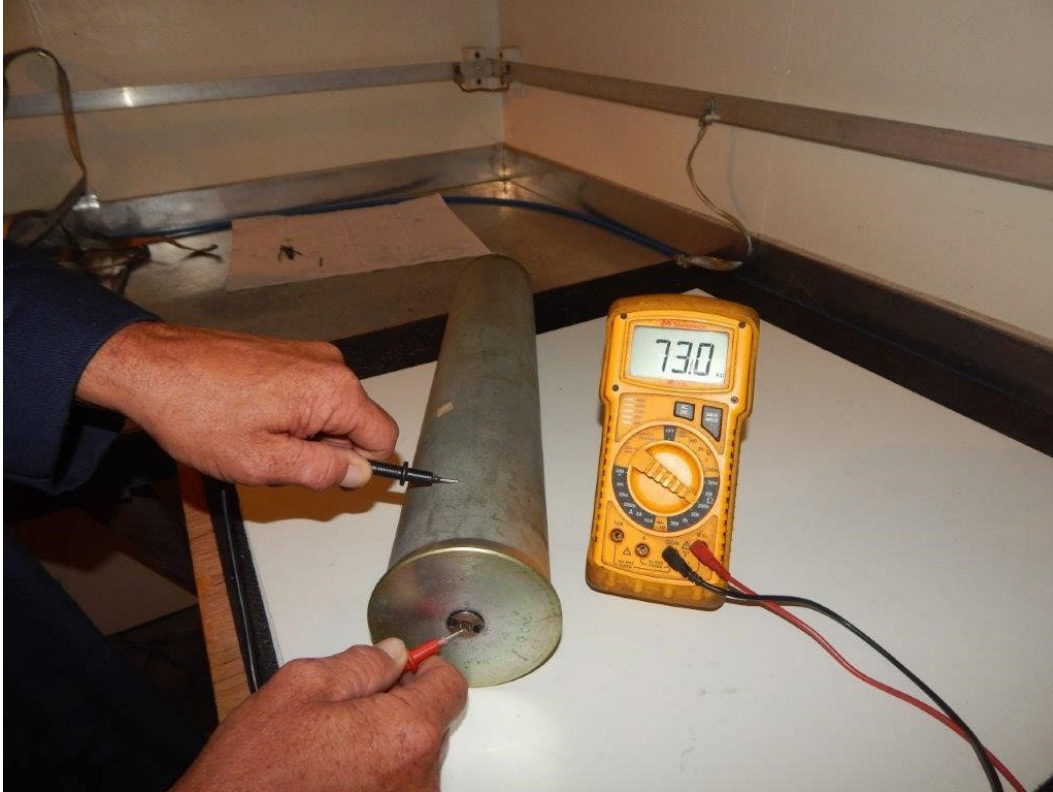
Fig. 15 Checking resistance of the primer through the case
