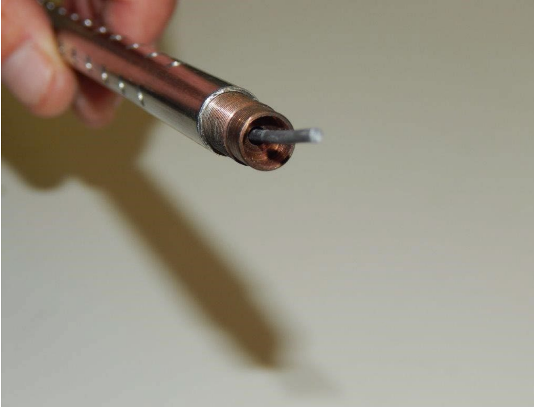
Fig. 10 Benite strand extended through primer housing
