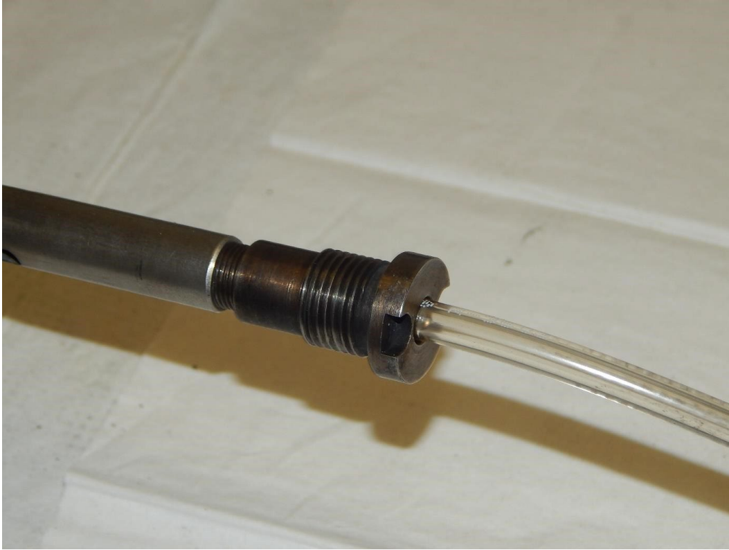
Fig. 12 Firing pin assembly threaded onto spit tube
