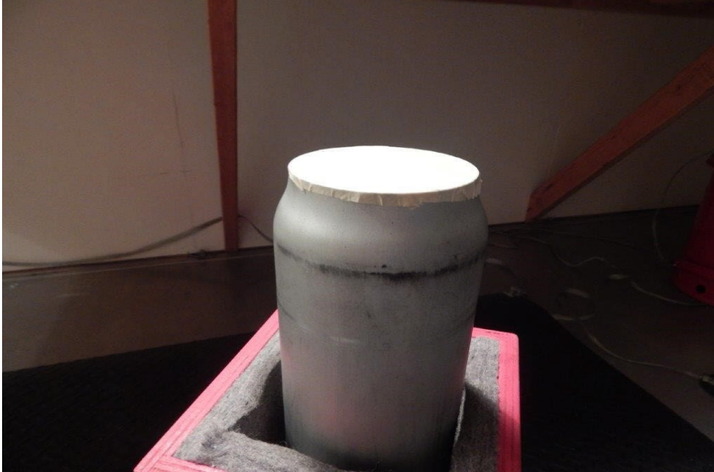
Fig. 19 Case covered with tape and trimmed
