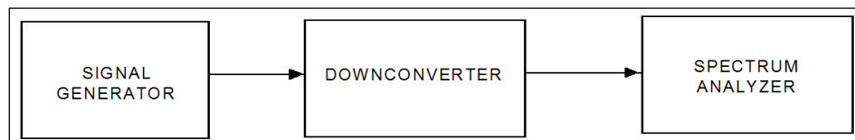
Figure 6-8. Downconverter Spurious Signal Generation
