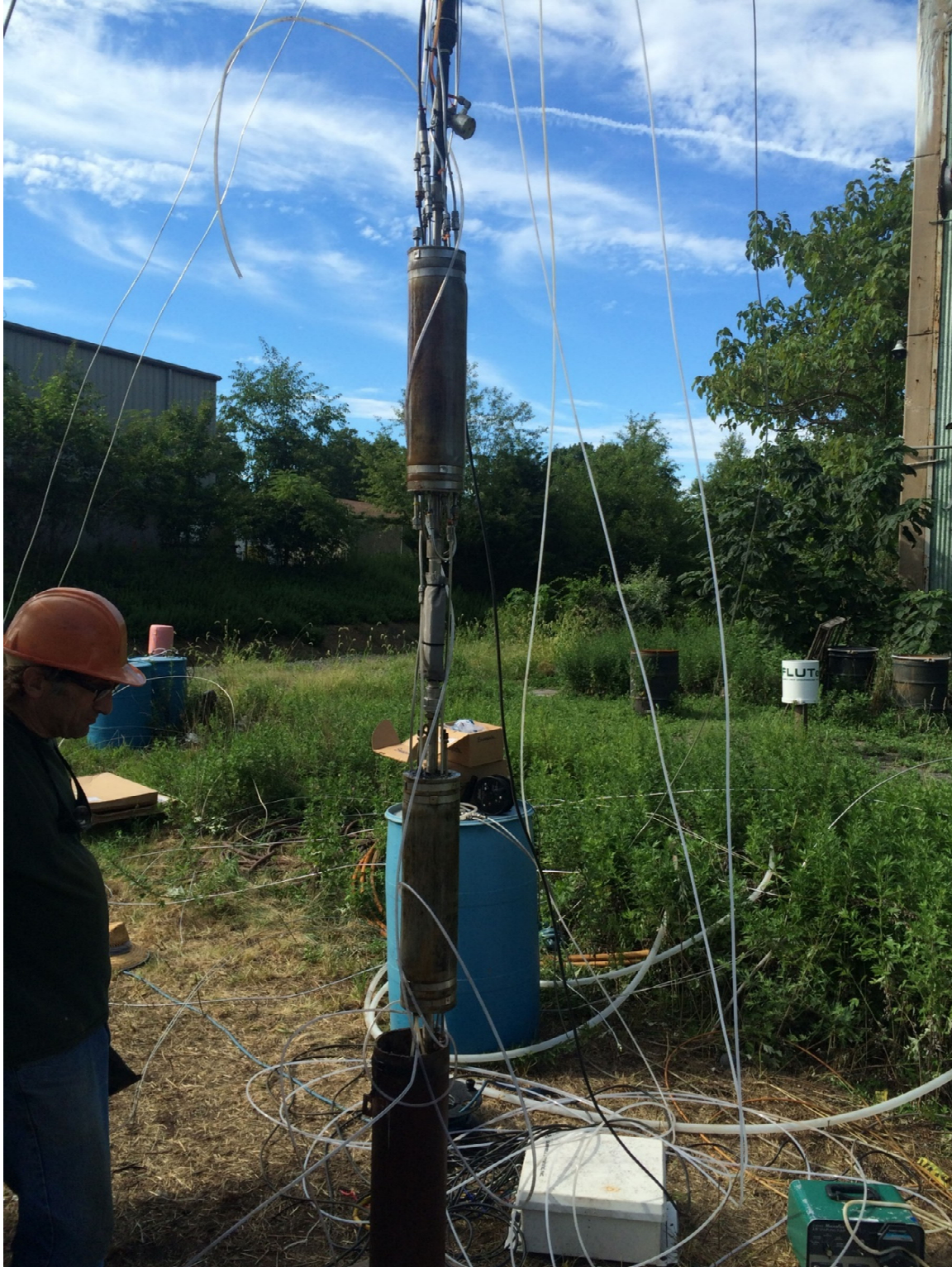
Figure 8. Custom-manufactured packer system being lowered into borehole for field testing. A microbial sampler (stainless-steel mesh bag containing inert sand support) is fixed in the test interval between the packers.
