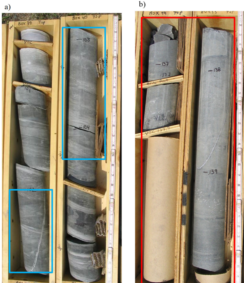
Figure 7. Photographs of selected rock core from 68BR. Blue box in (a) marks in GryMas-234 strata equivalent to the 71BR-85 test interval and red box in (b) marks rock core that are in GryMas-263 strata equivalent to the 07BR-49 test interval. Numbers represent approximate depths of core in situ, in feet. Image created by A. Fiore for this report.
