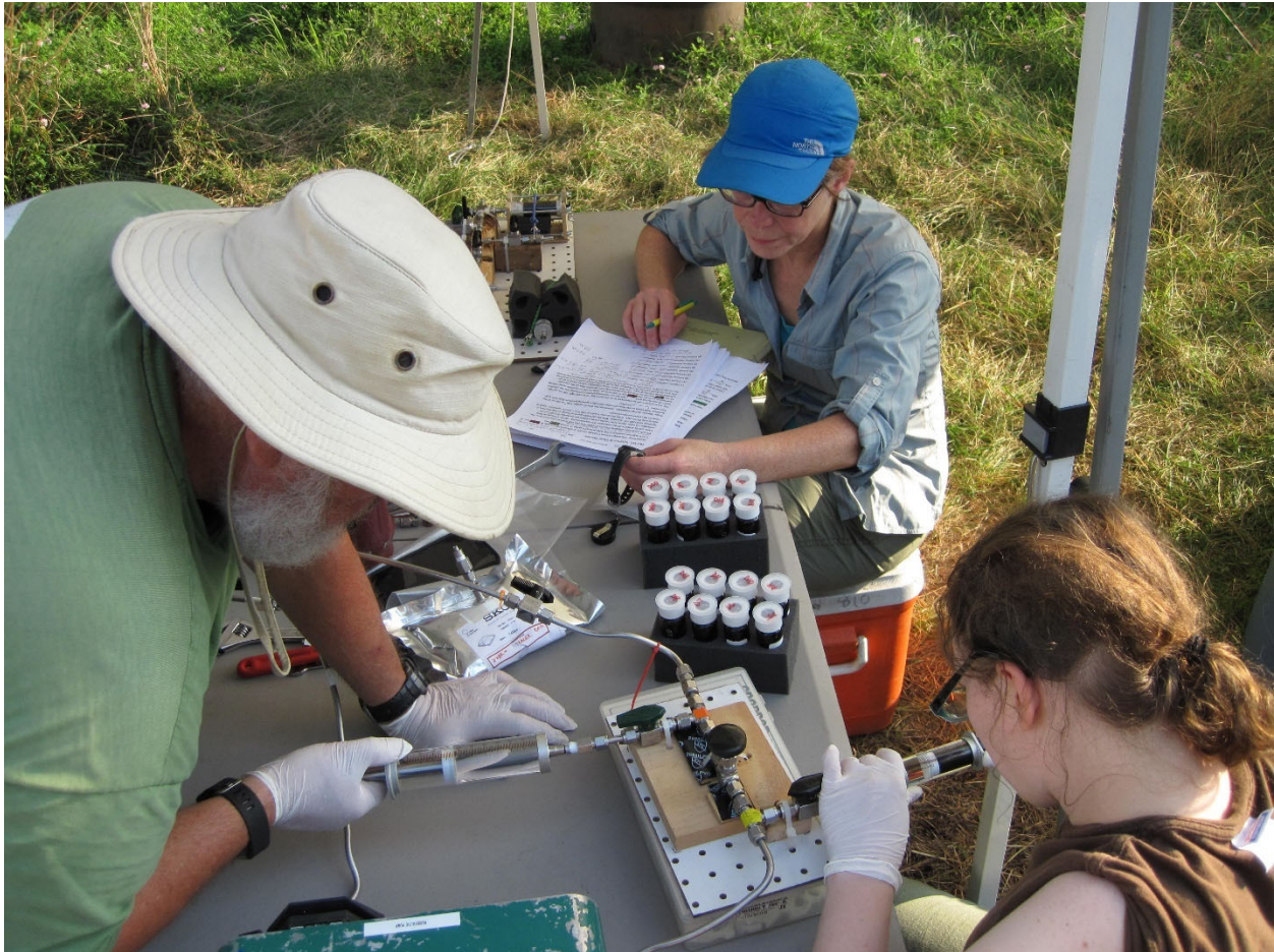
Figure 14. Dosing test interval without volume change by simultaneous injection of concentrated tracer solution into continuous flow (circulation from the test interval) and withdrawal of return flow.
