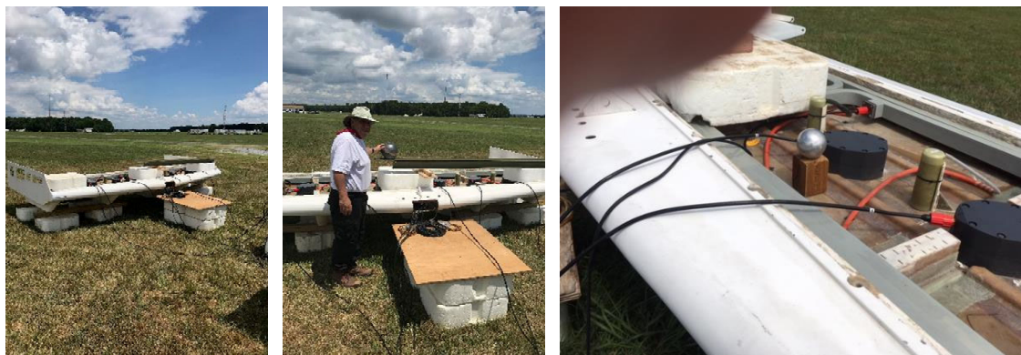
Figure 6. (left) MTA with EMI array installed, (center) Sphere rolling test, (right) Close-up of MTA showing magnetometers, receiver housings, and transmitter loops.
