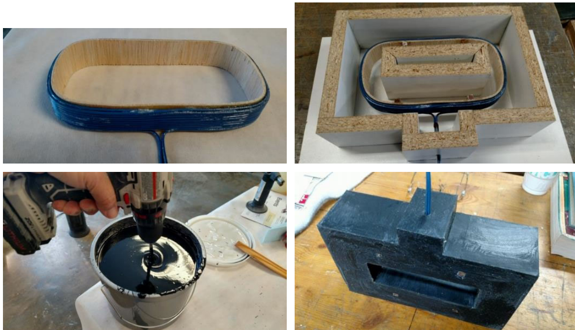
Figure 5. (upper left) Sample EMI coil winding, (upper right) Sample EMI coil suspended in form, (lower left) Waterproof epoxy being mixed, (lower right) Final sample coil released from mold.
