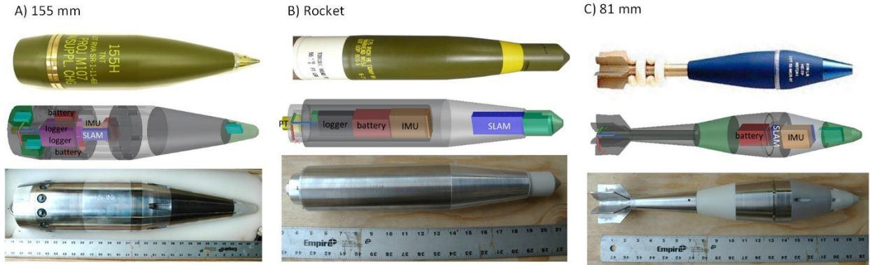
Figure 4. Example of munitions, CAD drawing, and fabricated surrogates for A) 155 mm Howitzer, B) Hydra 70 Rocket and C) 81 mm mortar. A ruler is provided for scale.
