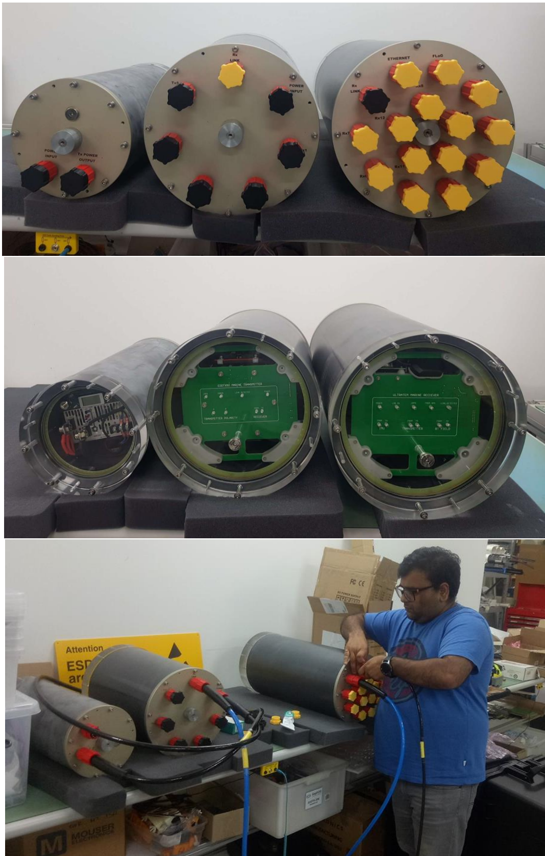
Figure 10. UltraTEM enclosures (from left to right they are power supply, transmitter & receiver)
