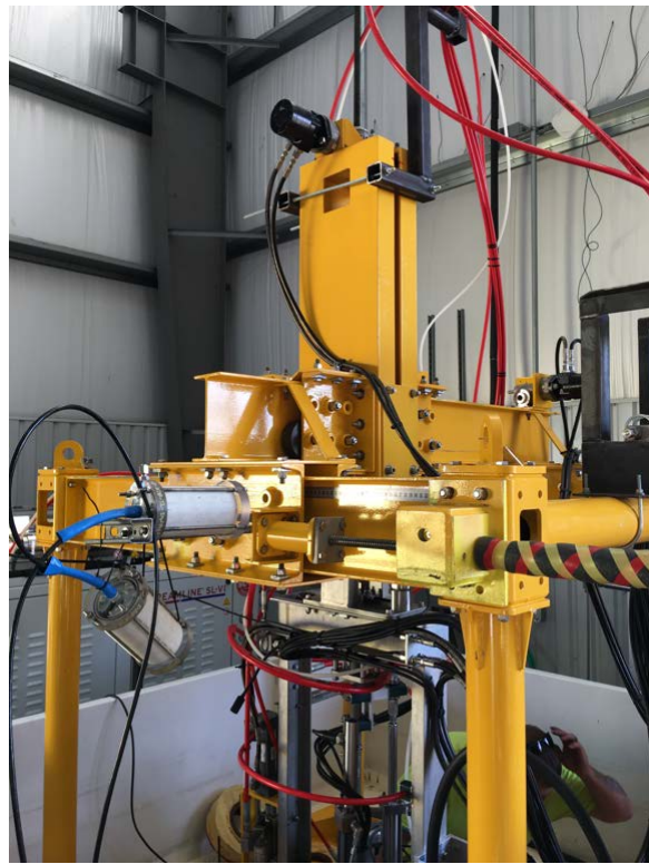
(d) Tool package gantry and high-pressure tube routing.
