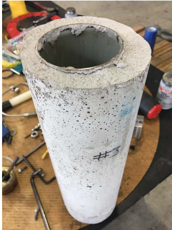
Figure 17: Concrete covered pipe for cleaning head testing.
