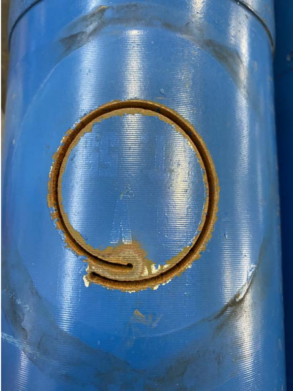
(a) Spiral cut resulting from motion of the cutting head relative to the projectile during testing.
