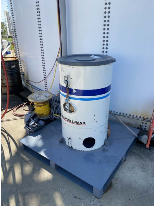
(a) Abrasive hopper positioned by the large test tank.
