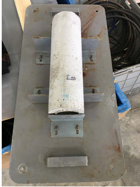
(a) Concrete covered pipe in cradle for processing.
