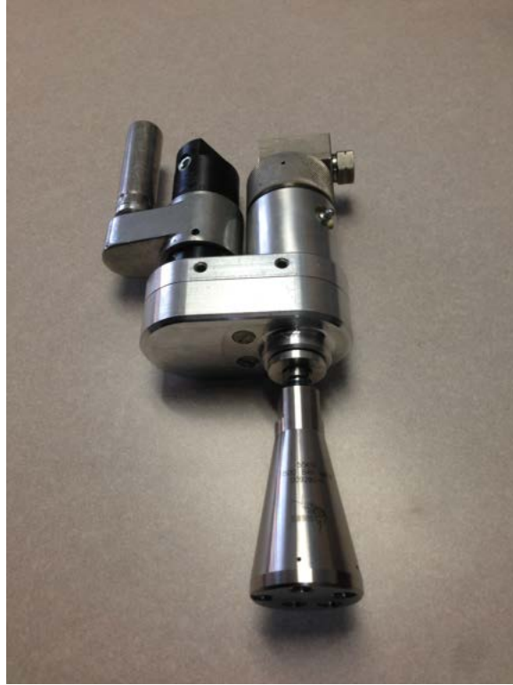
Figure 3: High-pressure waterjet cleaning tool.
