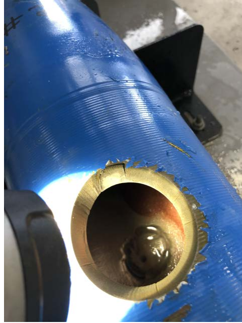
(b) Close view of the backside of the projectile after washout; notice some cutting of the backside material occurred.
