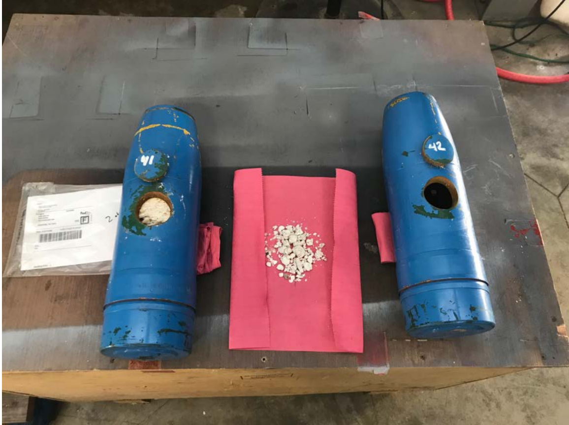
Figure 26: Inert filled projectiles after cutting/plug removal and washout.
