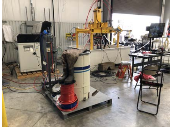
(b) Abrasive feed system, high-pressure intensifier, and tool package inside the shop test tank.
