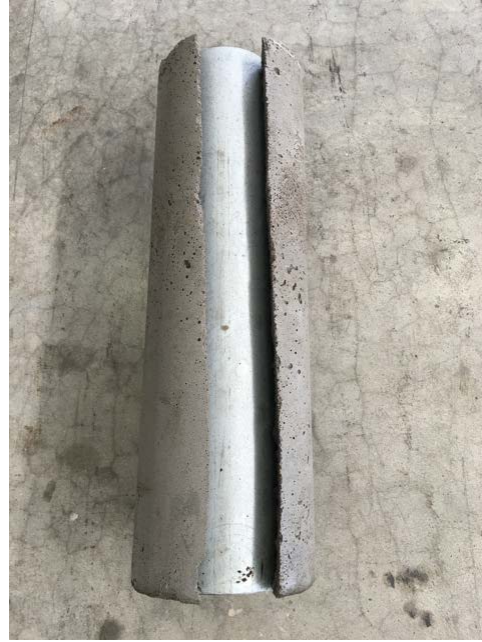
(b) Concrete covered pipe after cleaning underwater.
