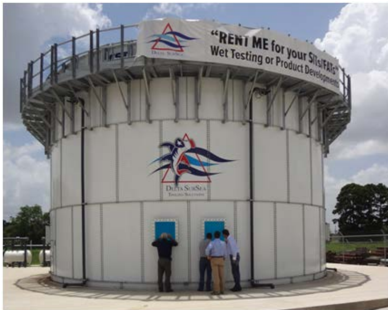
Figure 12: Delta SubSea’s tooling test tank that is 38.3 feet in diameter and 23.4 feet deep holding 200,567 gallons of water.
