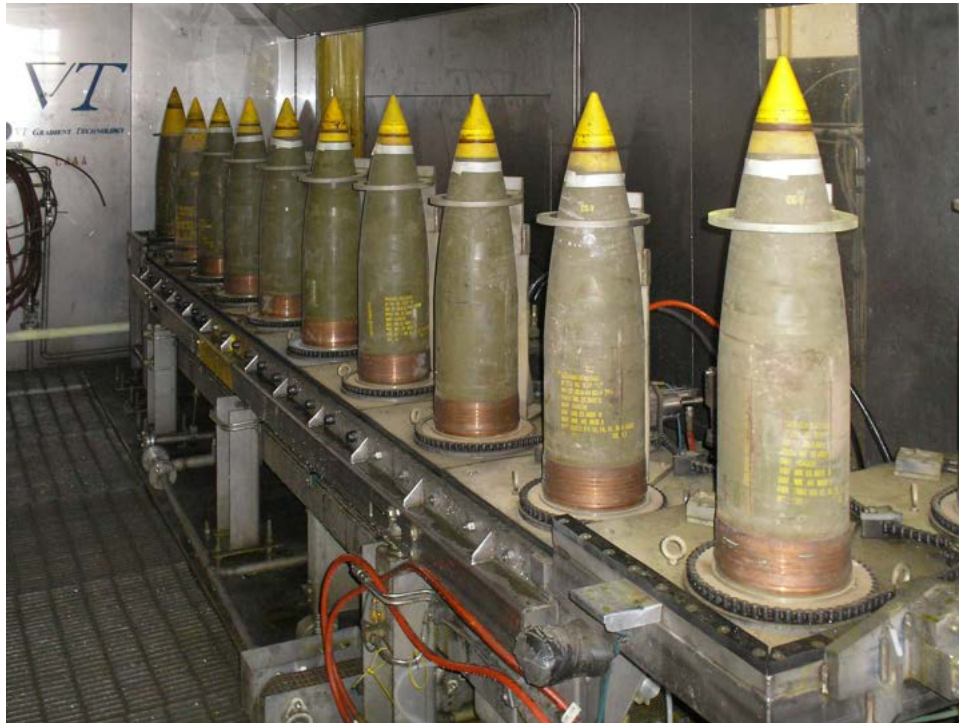
Figure ES 1: Automated AWJ cutting and washout system processing 8-in/55-cal HC rounds.
