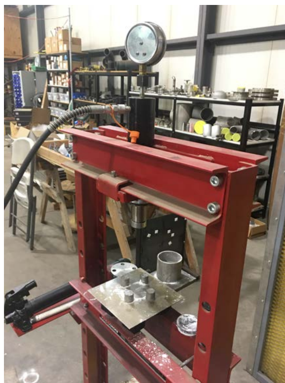
Figure 19: Hydraulic press for pressing the inert fill into the target items.
