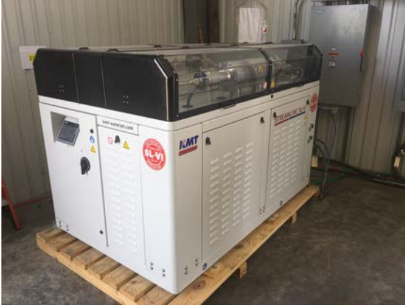
(a) KMT 100 hp high-pressure intensifier.
