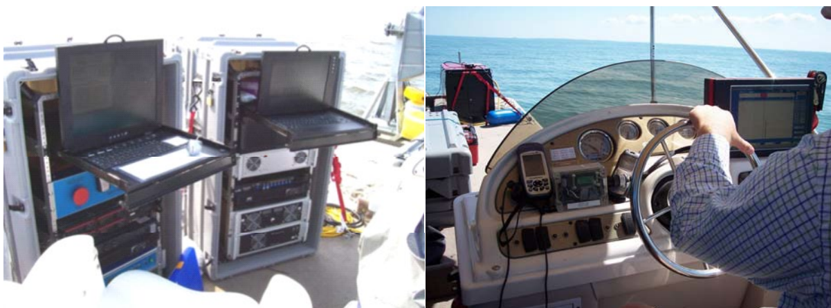
Figure 5-5. (Left) All Sensor Data Are Recorded by the Computers in These Data Racks Mounted Across from the Drive Console, near the Port Rail. (Right) The Tow Vessel Console Is Located on the Starboard Side. The Pilot Is Responsible for Maintaining the Survey Course and Avoiding Bottom Obstacles.
