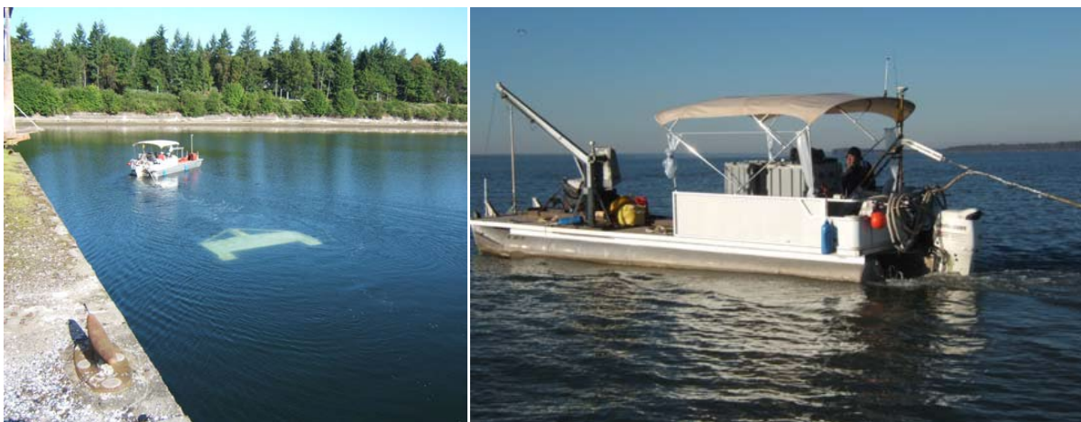
Figure 5-4. (Left) The 30 ft Pontoon Boat Is Shown Towing the Sensor Platform During a Survey on Ostrich Bay. The Sensor Platform Is Submerged About 7 ft. Below the Surface. (right) The Tow Point Fixture is Located at the Rear of the Boat. The master GPS antenna is located on the mast above this point. The digital angular encoder measures the angle of the tow cable relative to the boat heading. The weak link cable is located between the shackles at the end of the tow arm.
