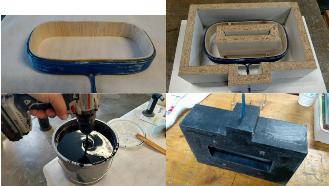
Figure 2-3. (Upper Left) Sample EMI Coil Winding, (Upper Right) Sample EMI Coil Suspected in Form, (Lower Left) Waterproof Epoxy Being Mixed, (Lower Right) Final Sample Coil Released from Mold.
