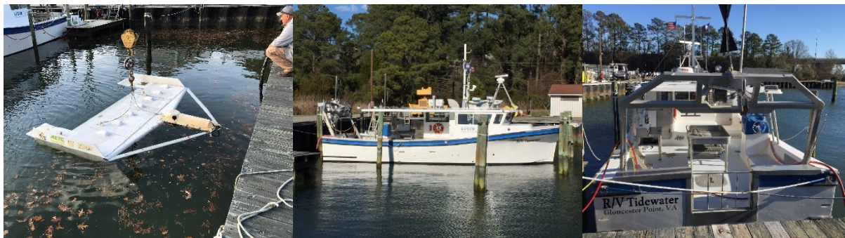
Figure 5-7. (Left) Marine Towed Array During a Float Test at VIMS, (Center) R/V Tidewater, and (Right) R/V Tidewater aft Lift.
