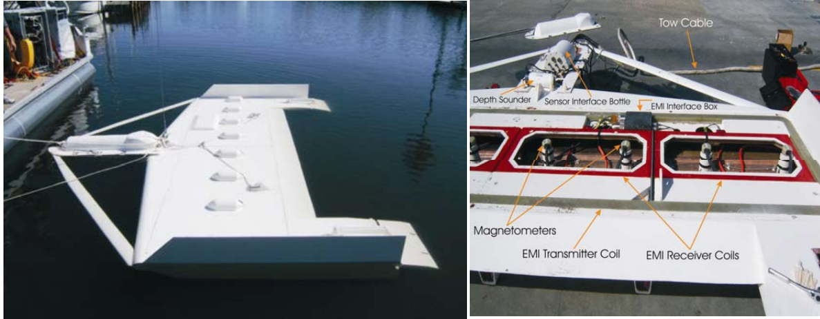
Figure 5-6. (Left) The Assembled Sensor Platform Is Shown, (Right) The Marine Sensor Platform Is Shown with the Hatch Covers Removed.
