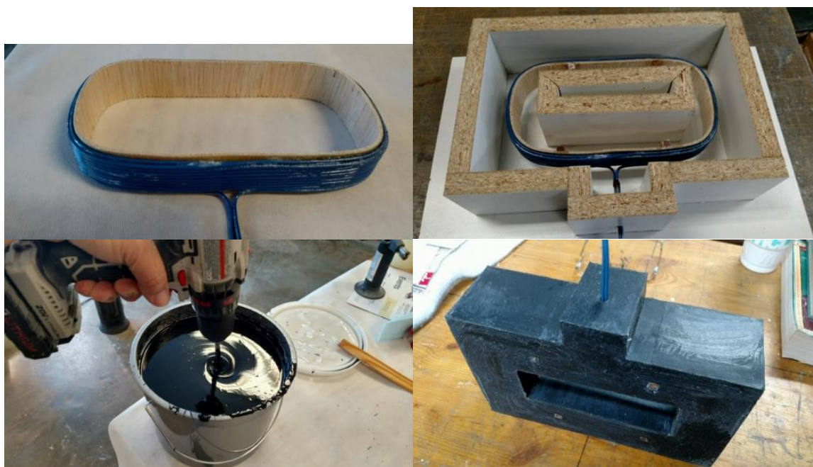
Figure E-2. (Upper Left) Sample EMI Coil Winding, (Upper Right) Sample EMI Coil Suspended in Form, (Lower Left) Waterproof Epoxy Being Mixed, (Lower Right) Final Sample Coil Released from Mold.
