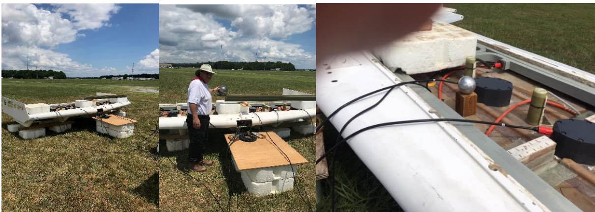
Figure 2-8. (Left) MTA with EMI Array Installed, (Center) Sphere Rolling Test, (Right) Close-up of MTA Showing Magnetometers, Receiver Housings, and Transmitter Loops.
