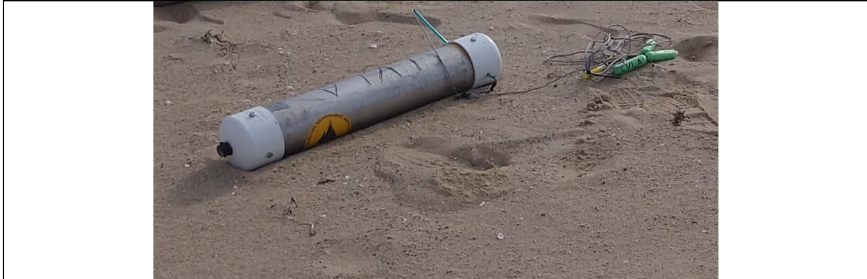
Figure 9. Surrogate UXO. The light and pressure sensor can be seen on the near end of the sUXO and the tether and small buoy on the far end.
