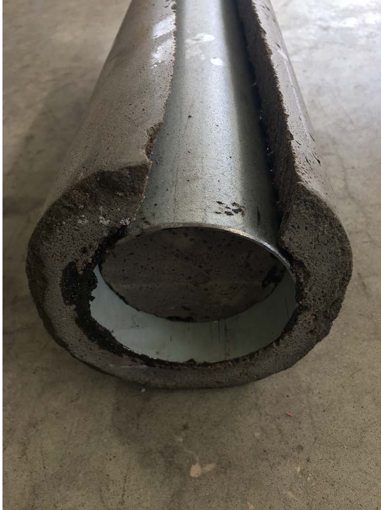
Figure 10. Concrete-covered inert target item after partial cleaning.
