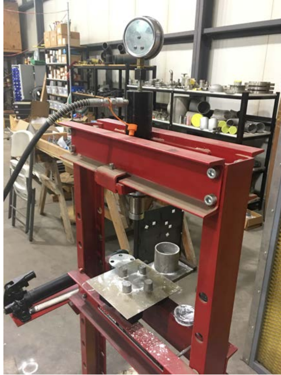
Figure 20. Hydraulic press for pressing the inert fill into the target items.
