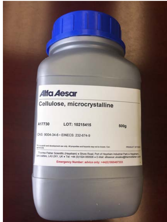
Figure 19. Microcrystalline cellulose to be used as the inert fill in the target items.
