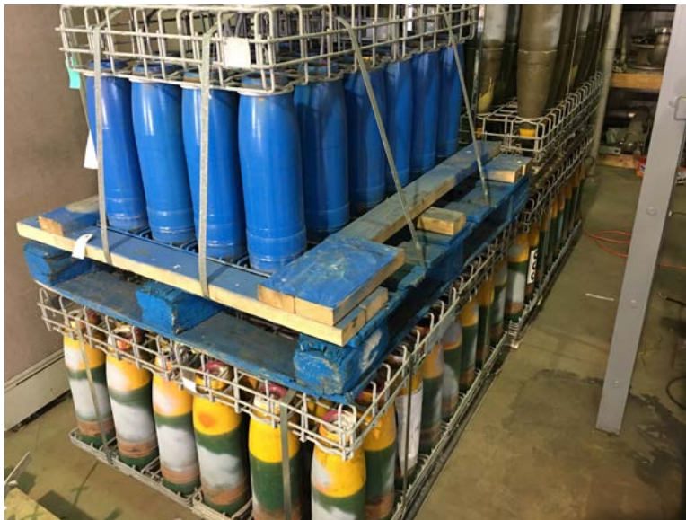
Figure 18. Demilitarized Navy 5-inch/38-caliber projectiles that will be used for target item creation.
