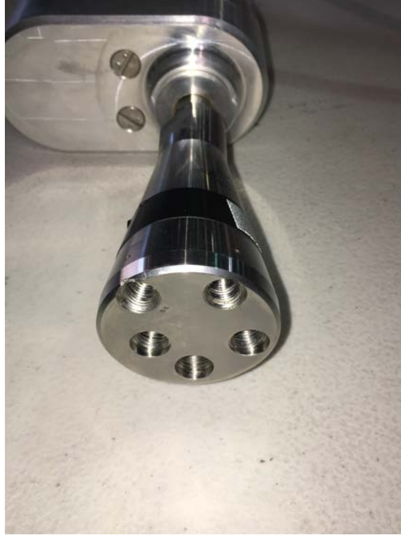
Figure 22. Cleaning head showing the five orifice positions.
