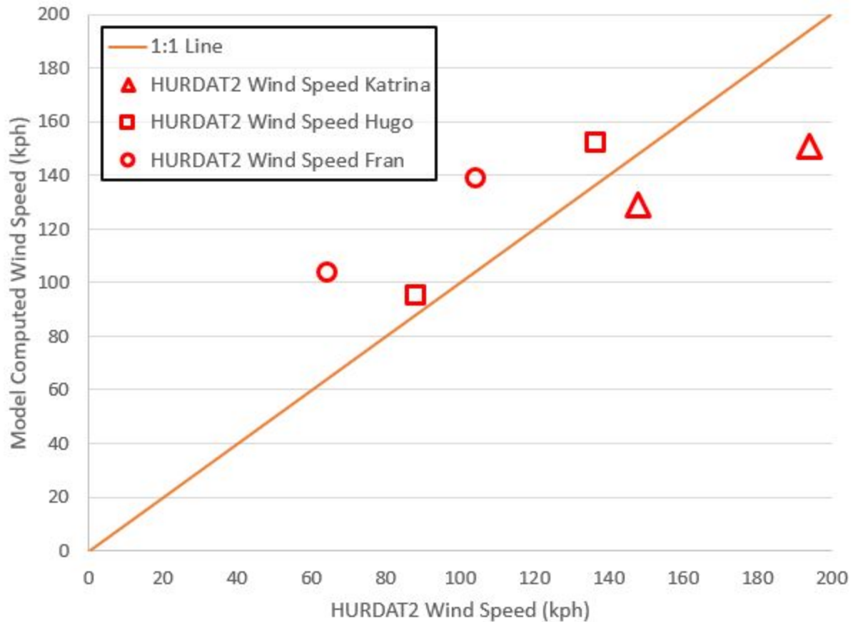
Figure 3: Comparison plot of Wind Speeds showing Measured and HURDAT2 values against Model computed values.
