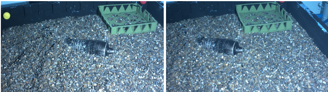
Figure 6.2: Stereo image pair from UW School of Oceanography test tank showing the simulated UXO in situ in the testbed.
