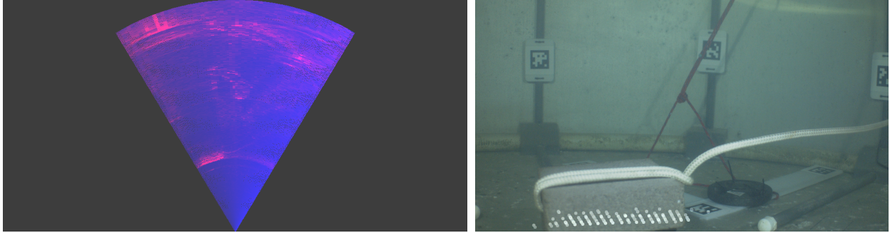
Figure 4.4: Sonar projection 2. This sonar projection shows the cinder block represented as a planar target in the sonar field of view, which is projected to the approximate correct location in the optical field of view.
