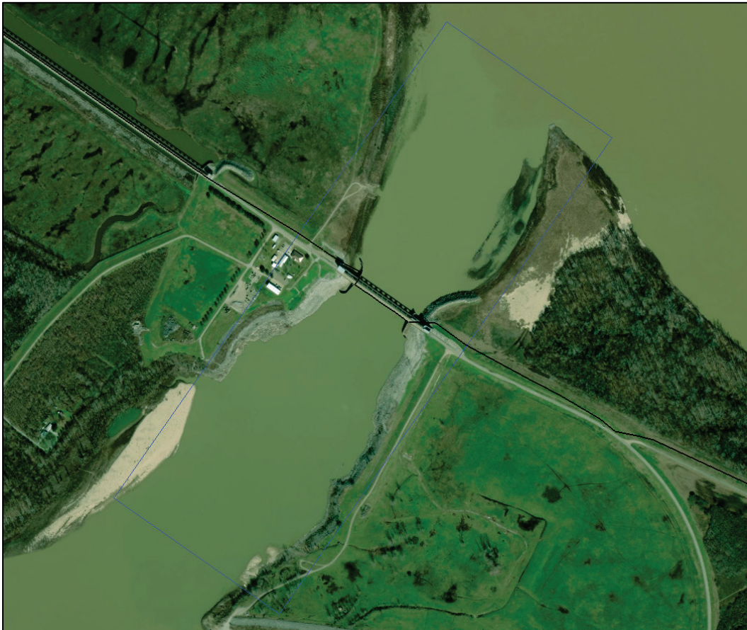
Figure 21. Physical model bounding box (flow splits were provided at the upstream locations).
