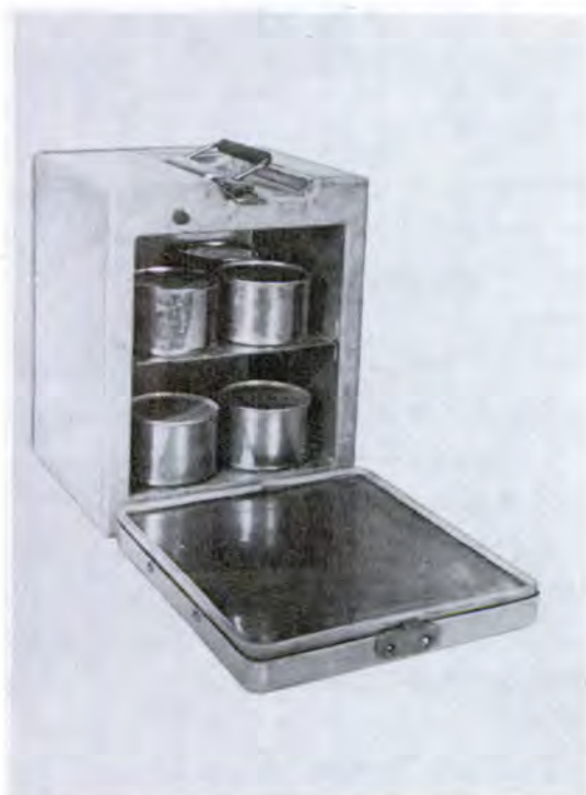
Figure 13-12. B-3 Oven With IF-Food Packet Cans in Place for Heating.
