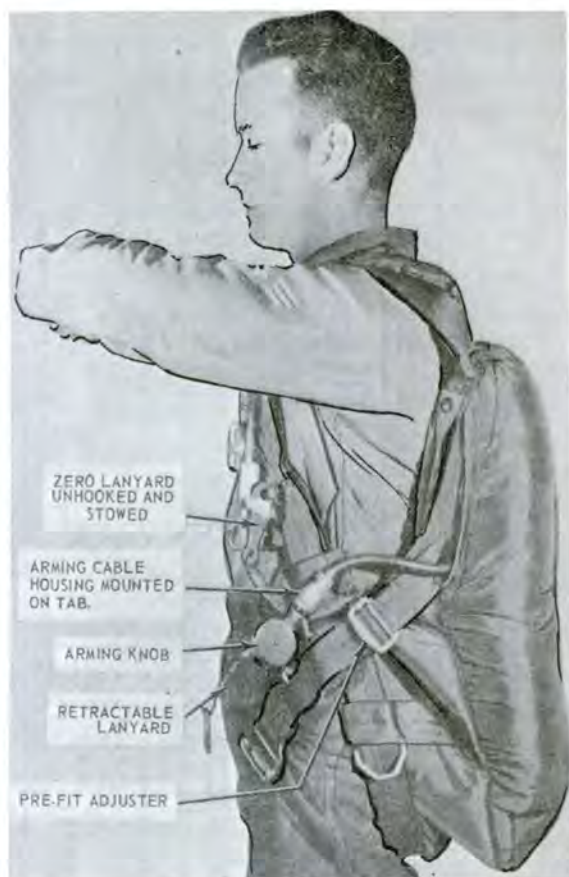
Figure 16-5. Arrangement of Arming Accessories, Automatic Back Parachute.
