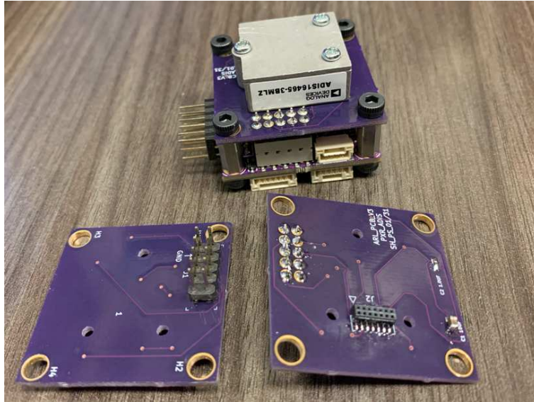
Fig. 8 The daughterboard top (right), bottom (left), and assembled with Pixracer R15 (top)
