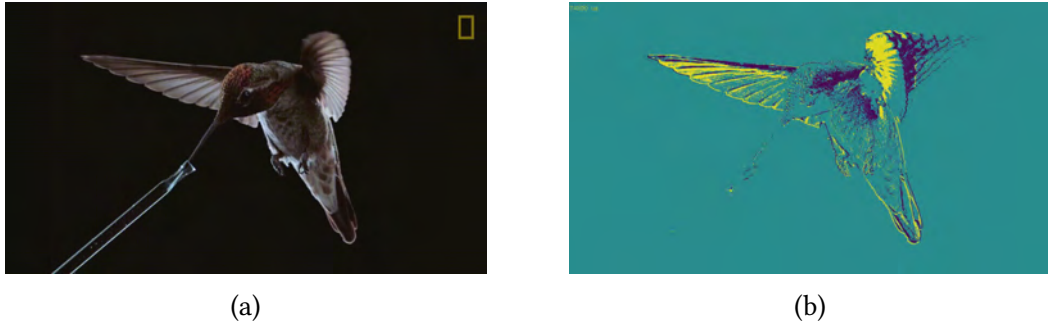
Figure 2: (a) Sample frame from the slow-motion video and (b) time surface rendered from simulated events using IEBCS.
