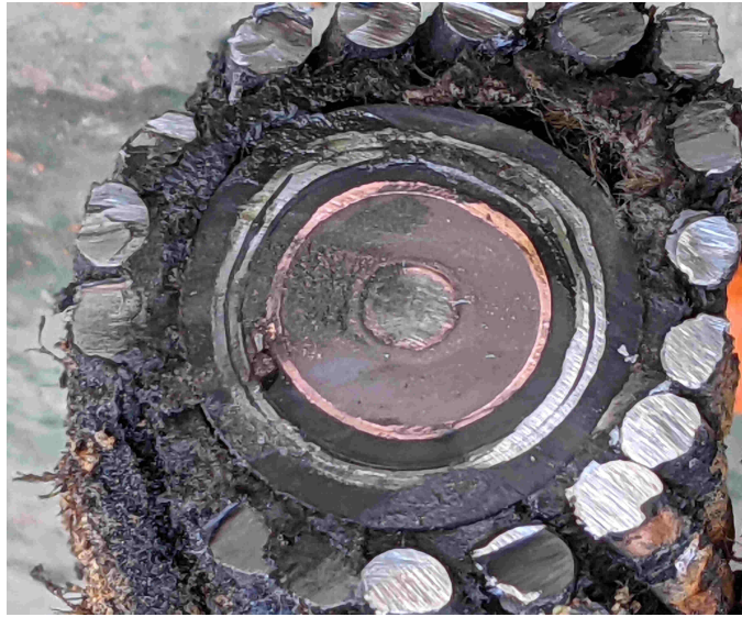
Figure 20: Cross-sectional view of the BSUREB77 shore cable.
