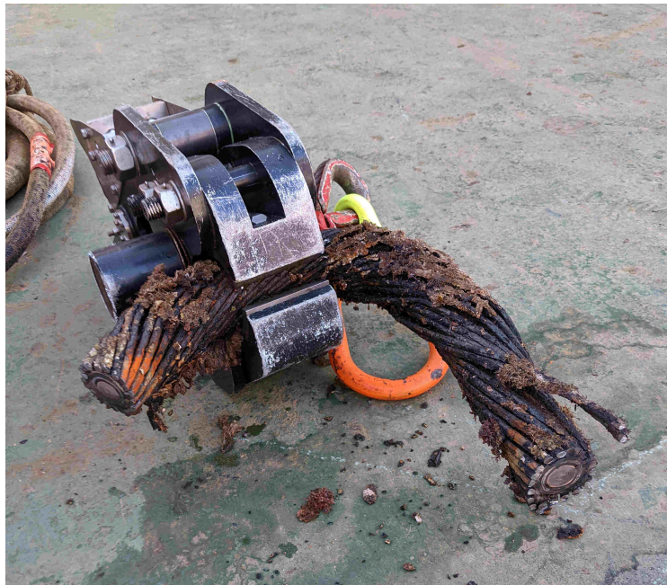
Figure 19: ROV gripper recovered onto the deck, after the BSUREB77 cable has been cut away. The gripper at maximum opening was just barely able to grab the cable (which is SDL5 cable, double armored.)
