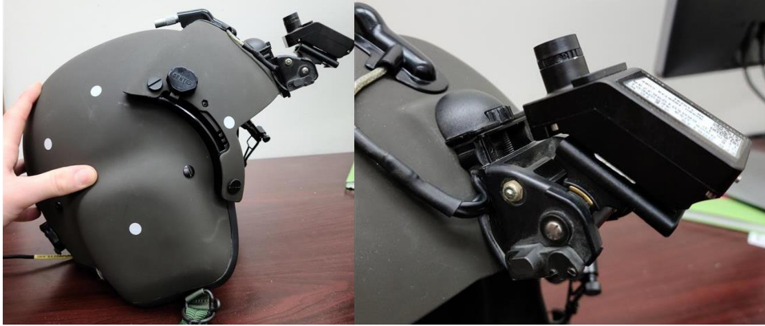
Figure 1. Gentex HGU-56/P flight helmet with the HOBIT attached to the night vision goggle mount.
