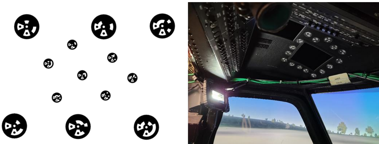
Figure 2. (Left) An example of the fiducial markers used by the HOBIT. (Right) A fiducial constellation installed in the flight simulator.
