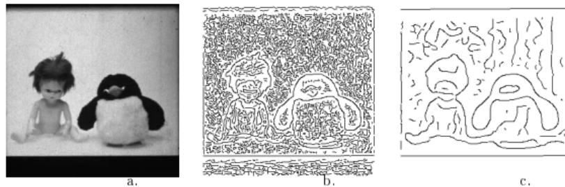
Figure 1: An example of edge detection, a type of image processing method. A) Original image, b) and c) images with two different max (1 and 4) gradients for detecting edges [7]
