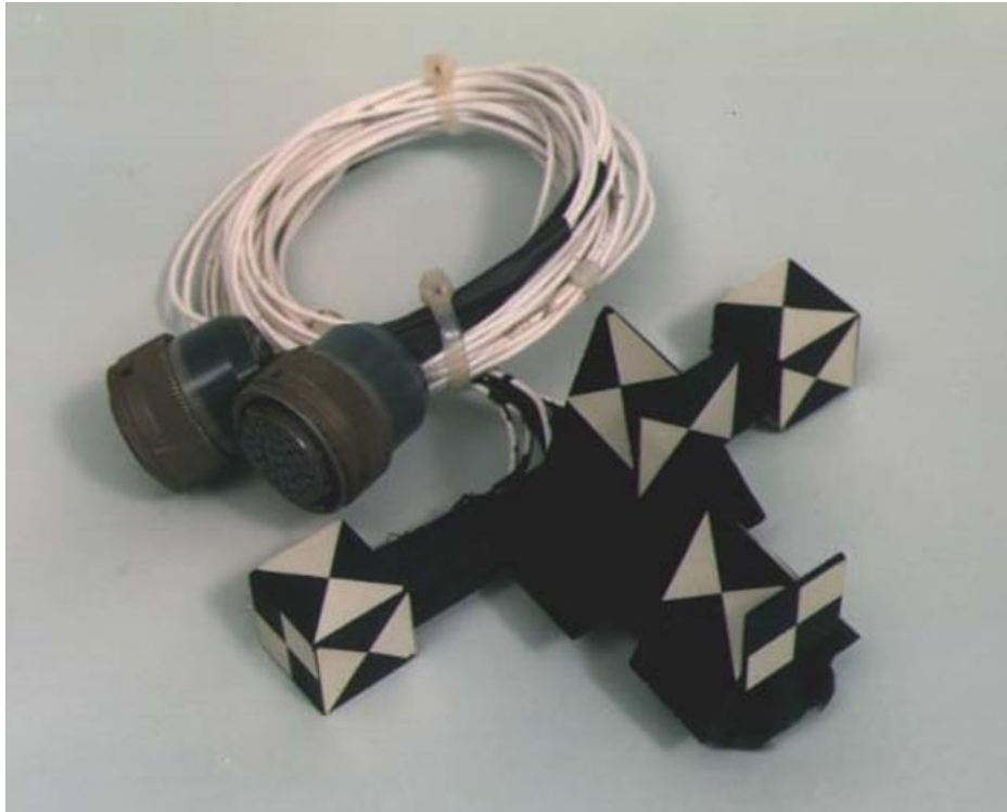
Figure 3. T-plate phototarget setup used to collect kinematic data from the high-speed film. The phototargets used for the T-plate and A-plate setups were similar, but, due to limitations of the subject size and test setup, the array configurations differed. The T-plate instrumentation was used for the chimpanzee subjects. See Appendix A for an example of the T-plate instrumentation on an HRV subject.
