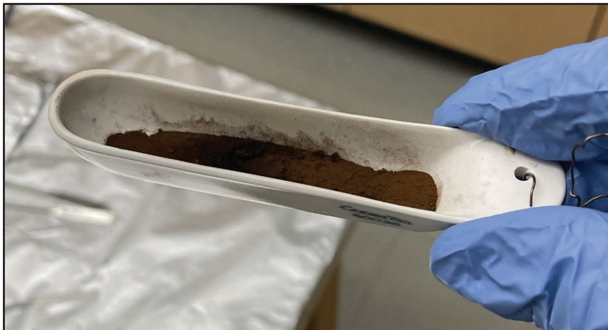
Figure 20: A photograph of the \text{Fe}_{25}\text{Ni}_{75} (20%) boat was taken shortly after reduction at 200 °C. The brown color seen across the majority of the sample is typical of no energetic event. The small blackened area in the middle of the boat is more typical of the powder resulting from an energetic event. Therefore, this composition was classified as a “partial” energetic event.
