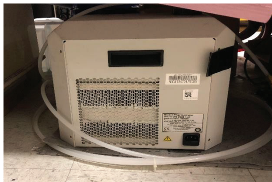
Figure 10.4: Cold water chiller for cool RB plate
