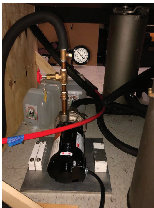
Figure 10.4: Cold water chiller for cool RB plate
