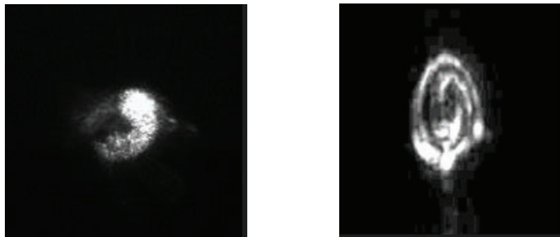
Figure 10: (a) FFI partially disintegrated by OT and (b) LG beam distorted by OT
