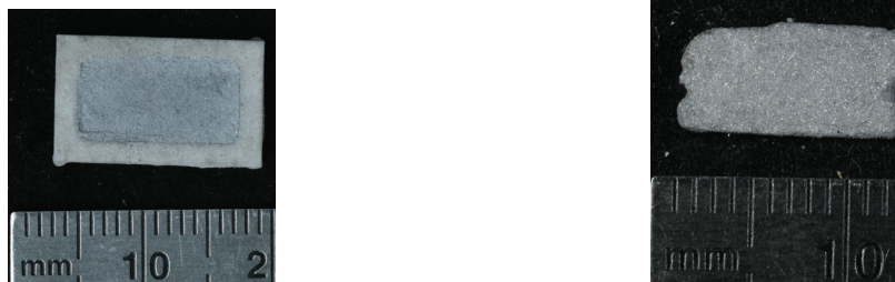
(a) 100 wt% Free Powder Sintering Sample in Mold (b) 100 wt% Free Powder Sintering Sample
