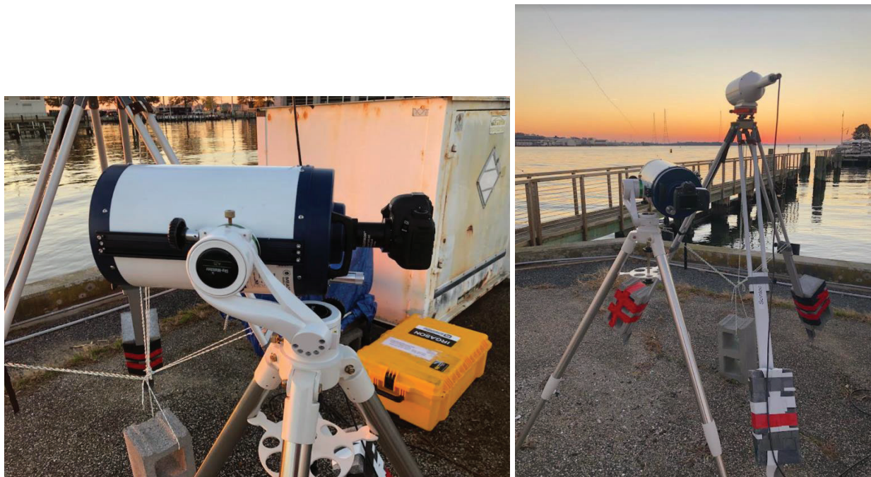
Figure 13: Initial experimental set-up; Canon EOS 5D Mark IV and Meade LX65 8" f/10 Optical Tube.
