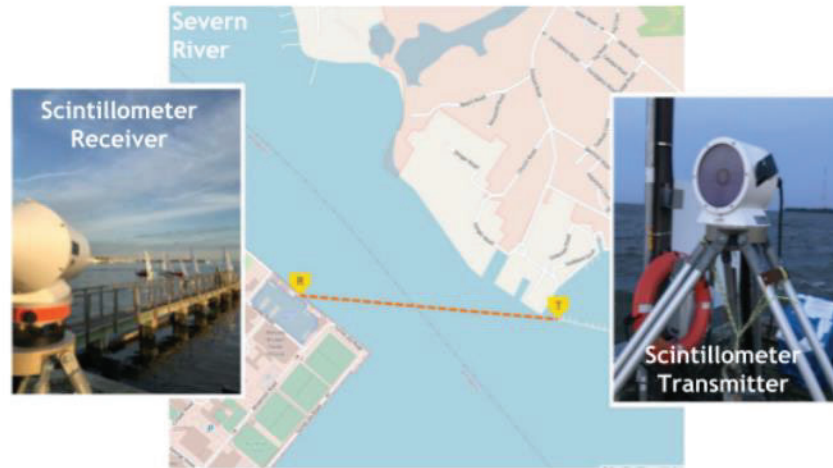
Figure 12: Location of scintillometer link over the Severn River. The camera field of view will encompass this same over water path [3].
