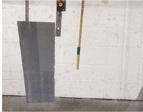
Figure 17: Millar sensor placed behind a half foil for wake detection.
