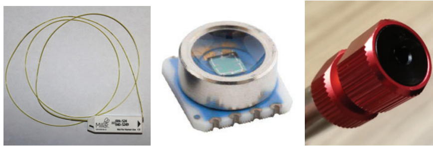
Figure 15: Pressure sensors considered for the lateral line. The Millar Microtip Pressure Transducer (left), Measurement Specialties MS5407-AM (center), and Blue Robotics Bar-02 (right).
