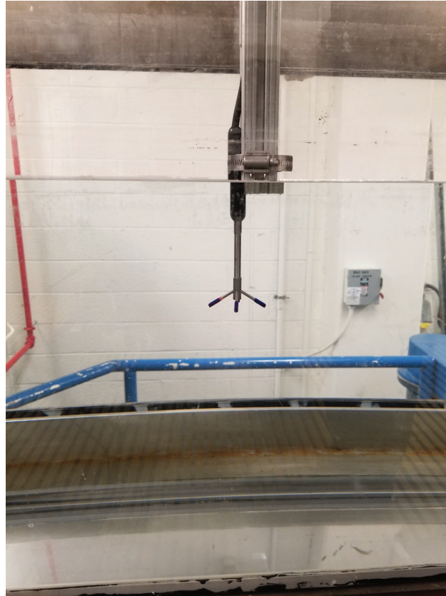
Figure 50: Acoustic-doppler velocimeter detecting exact tank speeds at various slow settings.
