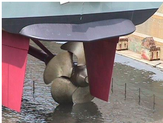
Figure 3. Stern Flap on DDG-51 Class Destroyer
