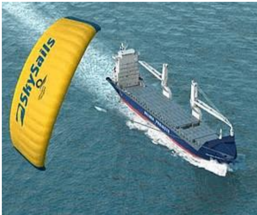
Figure 9. SkySails Concept Applied to Commercial Cargo Ship
