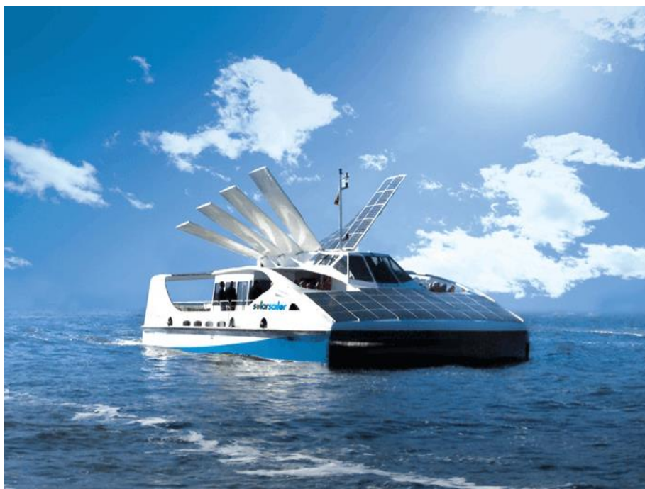
Figure 11. Solar Sailor Hybrid-Powered Ferry Boat
