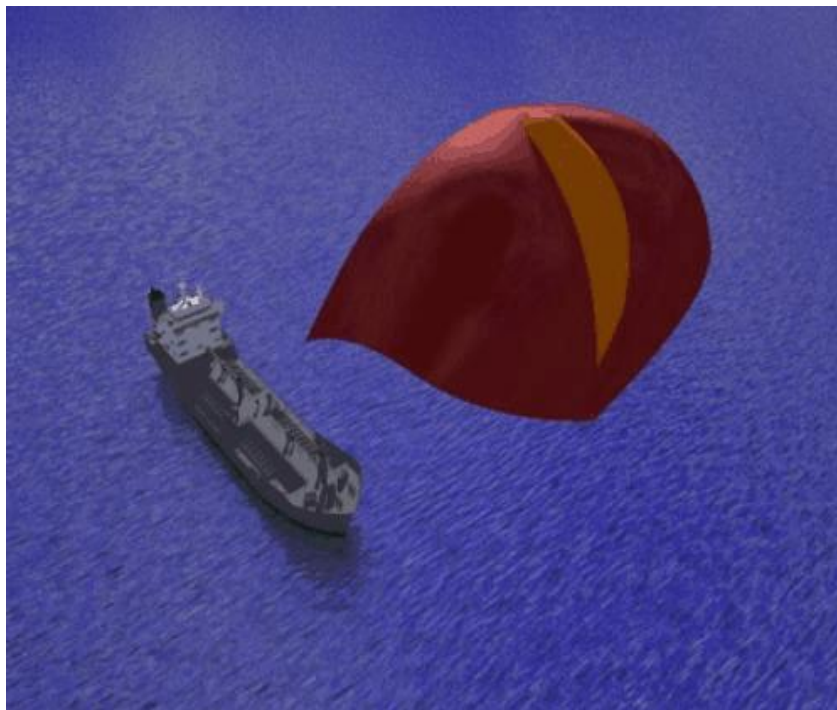
Figure 8. KiteShip Concept Applied to Commercial Cargo Ship
