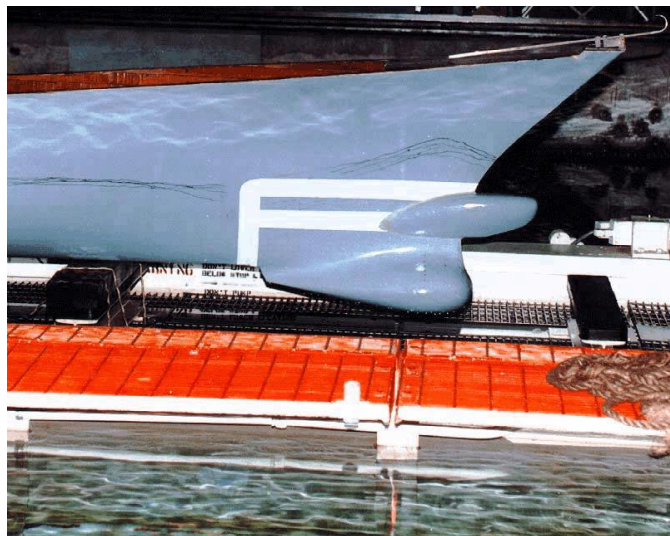
Figure 2. Bulbous Bow Design for DDG-51
