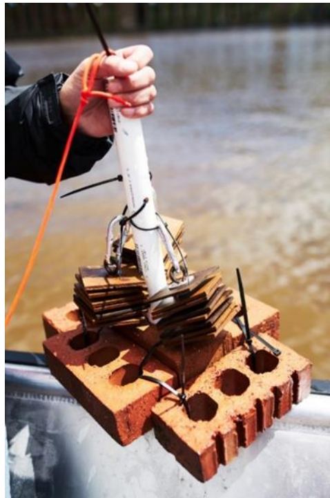
Figure 4. Hester Dendy (replicate units, as deployed in field).
