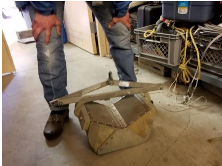
Figure 5. Ponar sampler to grab soft sediment samples.
