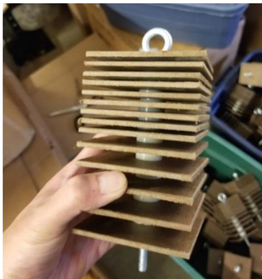
Figure 3. Hester Dendy (single unit).
