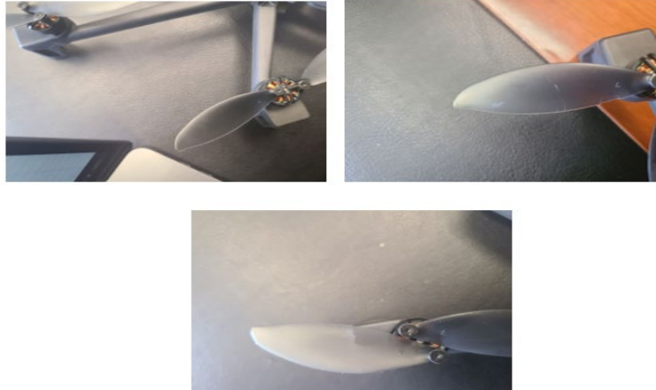
Fig. 5 Damaged propeller blades
