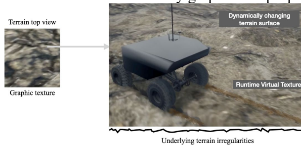
Fig. 5 Simulated vehicle traversing over one type of terrain representing low mobility determined by the graphical layer as something similar to mud, and by the physical layer with deformable properties.
