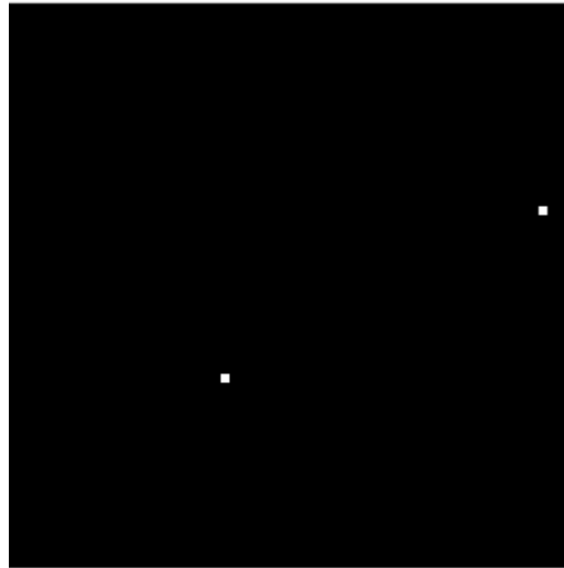
Figure 44. ROIC C2A01 during run 3 (frame 736, 78 MeV*cm 2 /mg, Tantalum). Two upsets can be observed (white pixels), but these errors do not persist to the next frame.
