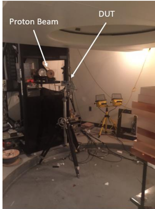
Figure 25. Test setup at the MGH Francis H. Burr Proton Beam Therapy Center.
