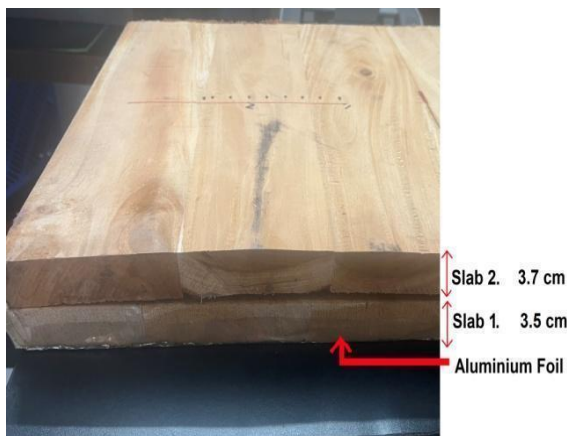
(c) Stacked arrangement of the wood sample for experiment
