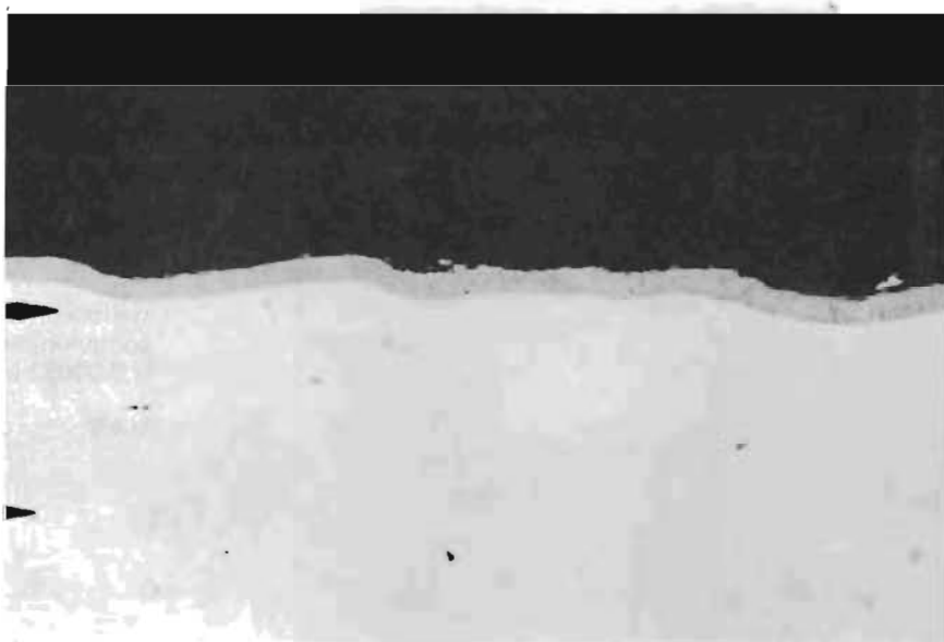
Figure 49. Inconel 600 - cross section comparison of control specimen and specimens exposed to hydrazine decomposition products for 10 hours at 1400° F.
