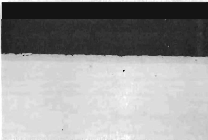
Figure 51. Inconel 718 - cross section comparison of control specimen and specimen exposed to hydrazine decomposition products for 10 hours at 1400°F.
