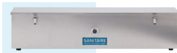
Figure 22. Sanitaire RSA760 ultraviolet air sanitizer draws air into the system using a fan, then passes the air over UVC lamps, which irradiates the air providing air disinfection for 3,800 cubic feet of space at 6 room air exchanges per hour. Source: BuyUltraviolet.com (n.d.).
