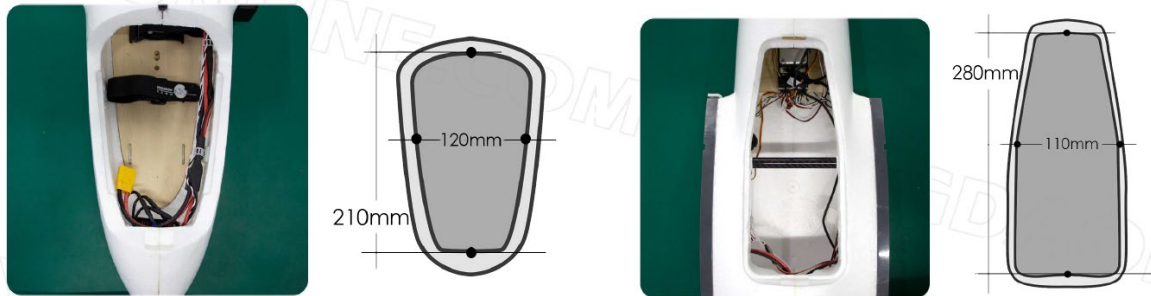
Figure 12. Battery dimensions. Source: [17].
