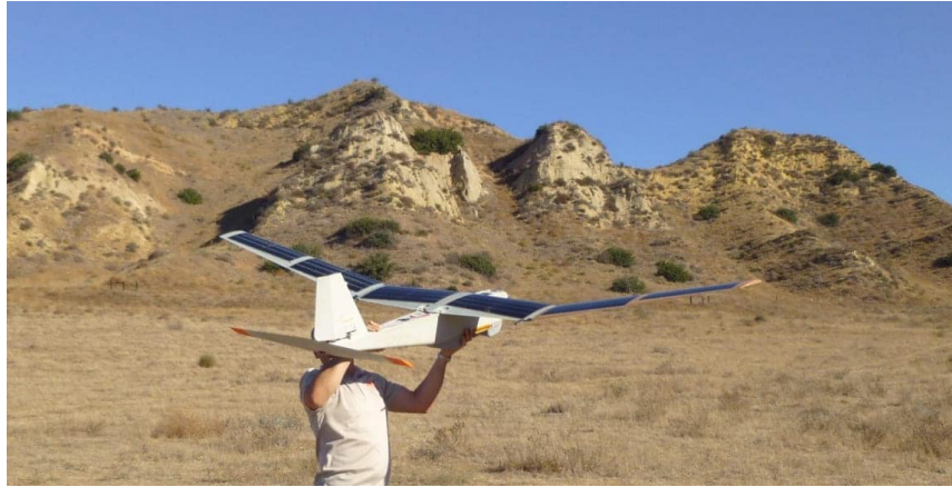
Figure 35. Silicon solar cells on UAV
