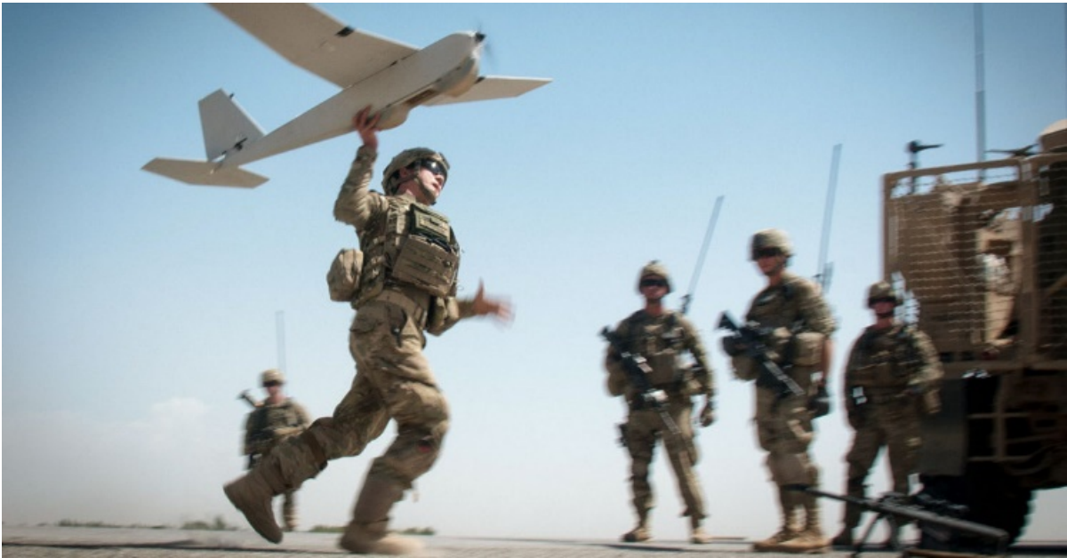
Figure 5. Launching the PUMA 3 AE
