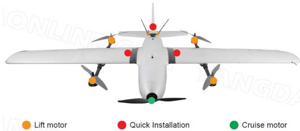
Figure 9. Nimbus Pro VTOL rotors and propellers. Source: [17].
