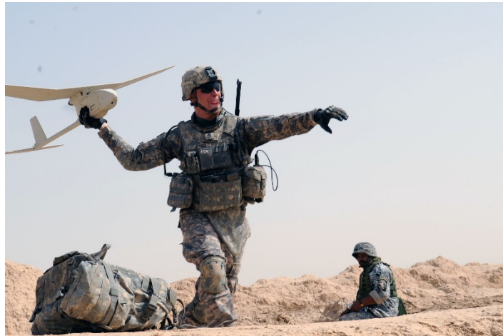
Figure 3. Launching the RAVEN RQ-11A/B
