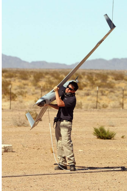
Figure 4. Launching a fixed-wing drone
