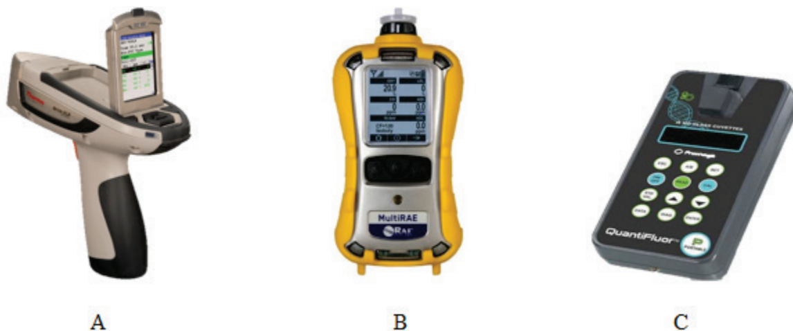
Figure 1. ETEO sensors, including A) XRF, B) gas monitor, and C) fluorometer.
