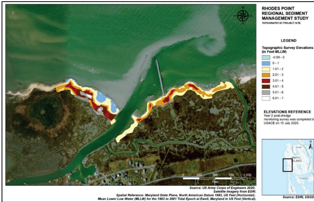
Figure 16. Topographic survey elevations from July 2020. Note the sediment plume coming off the placement site as the base image was taken prior to planting of the placement site in June 2019.
