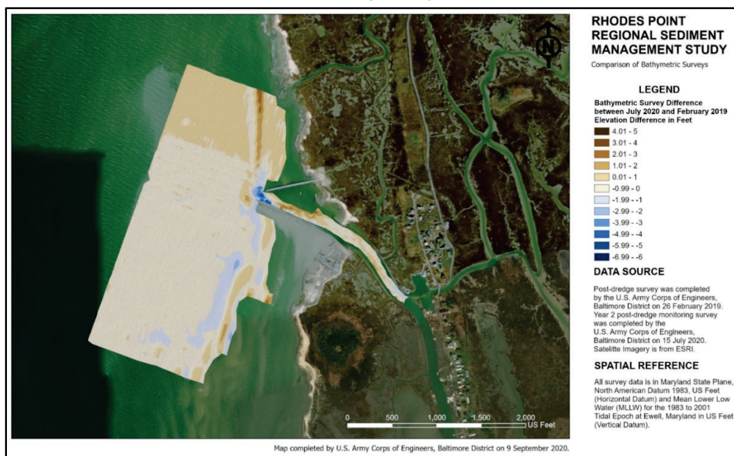
Figure 8. Comparison of bathymetric surveys for February 2019 and July 2020 showing elevation difference between surveys (negative denotes increased depth or erosion/scour).
