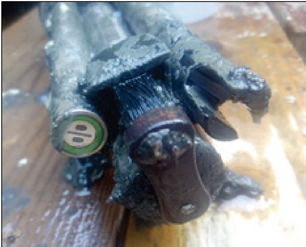
Figure 24. Biofoul on the reference area water quality sonde; however, the wiper kept the turbidity probe (left) clean during the deployment.
