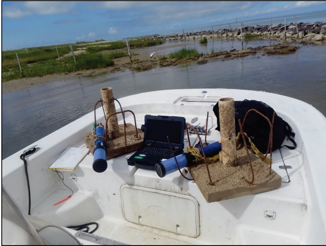
Figure 7. The two water quality sondes attached to concrete stands.
