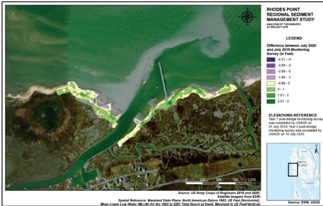
Figure 17. Differences in topographic survey between July 2019 and July 2020. Note the sediment plume coming off the placement site as the base image was taken prior to planting of the placement site in June 2019.
