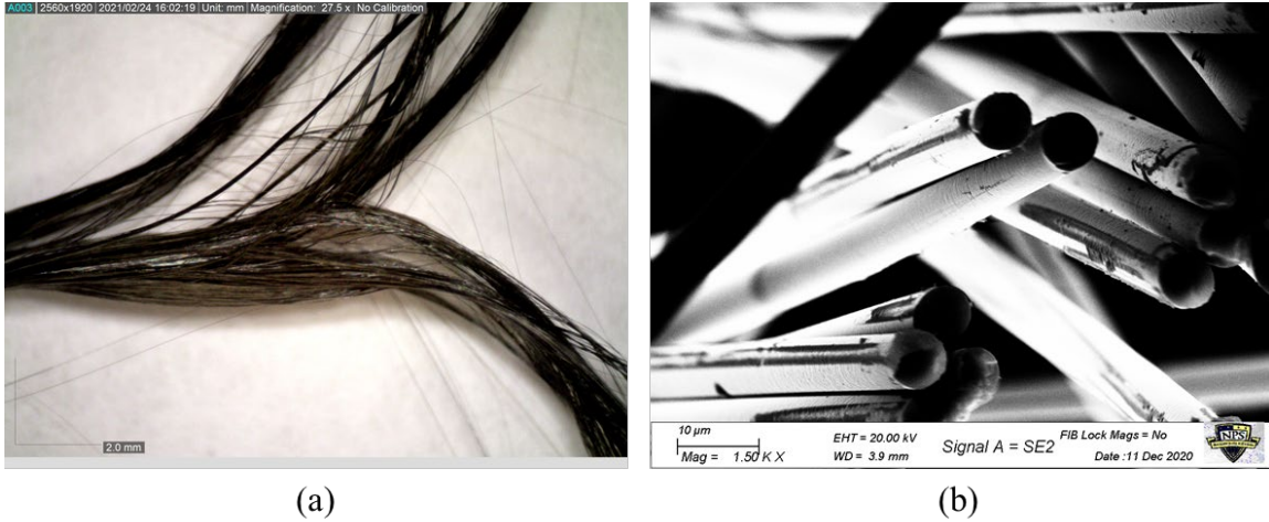
Figure 18. Tangled Fibers within a Fiber Bundle, (a) Optical Microscopy, (b) Scanning Electron Microscopy
