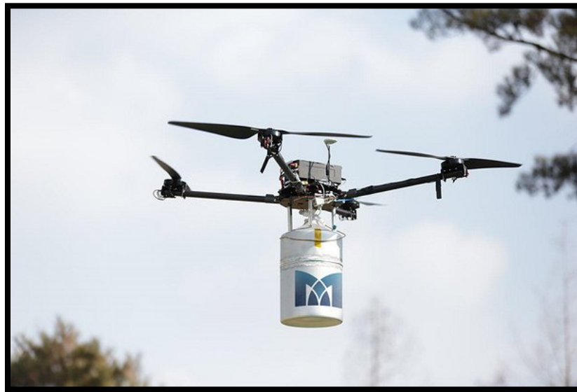
Figure 4. MetaVista's UAV Using 390 Grams of Liquid Hydrogen. Source: Inside Unmanned Systems (2019).
