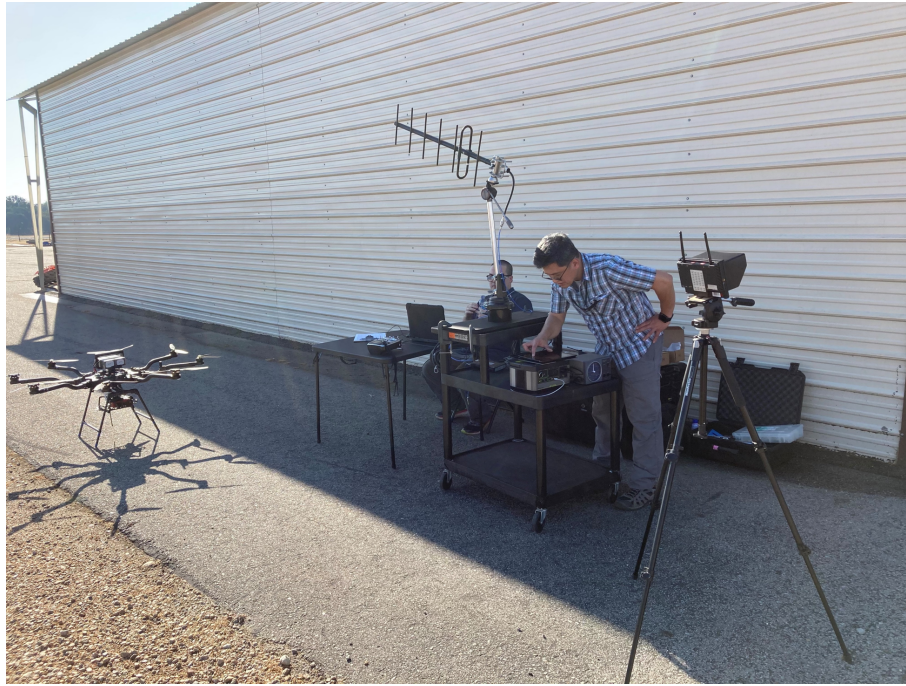
Figure A.7. Setup for experiments 4-6: receiver antenna at 24^\circ inclination page 2
