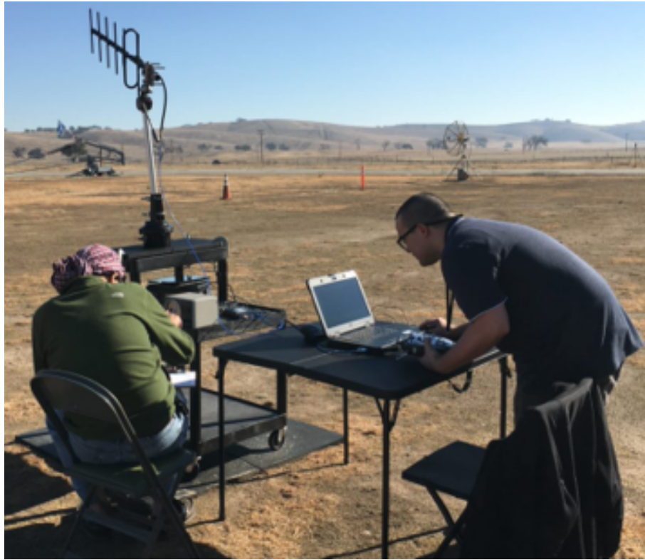
Figure A.6. Setup for experiments 4-6: receiver antenna at 24^\circ inclination
