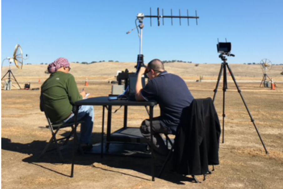
Figure A.5. Setup for experiments 1-3: receiver antenna at 0^\circ inclination
