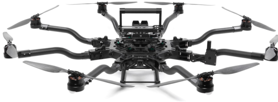
Figure 5.2. Freefly Alta 8 drone. Source: [16].
