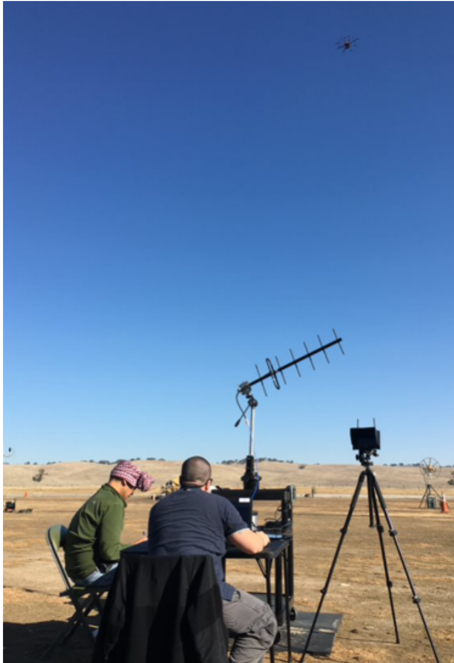
Figure A.8. Setup for experiments 4-6: receiver antenna at 24^\circ inclination page 3
