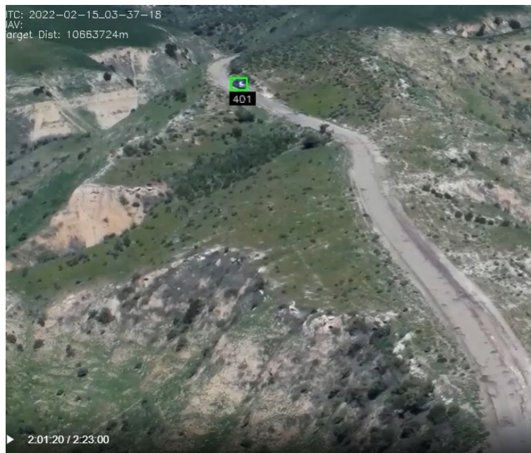
Figure 17. Maximum Range of Vehicle Detection
