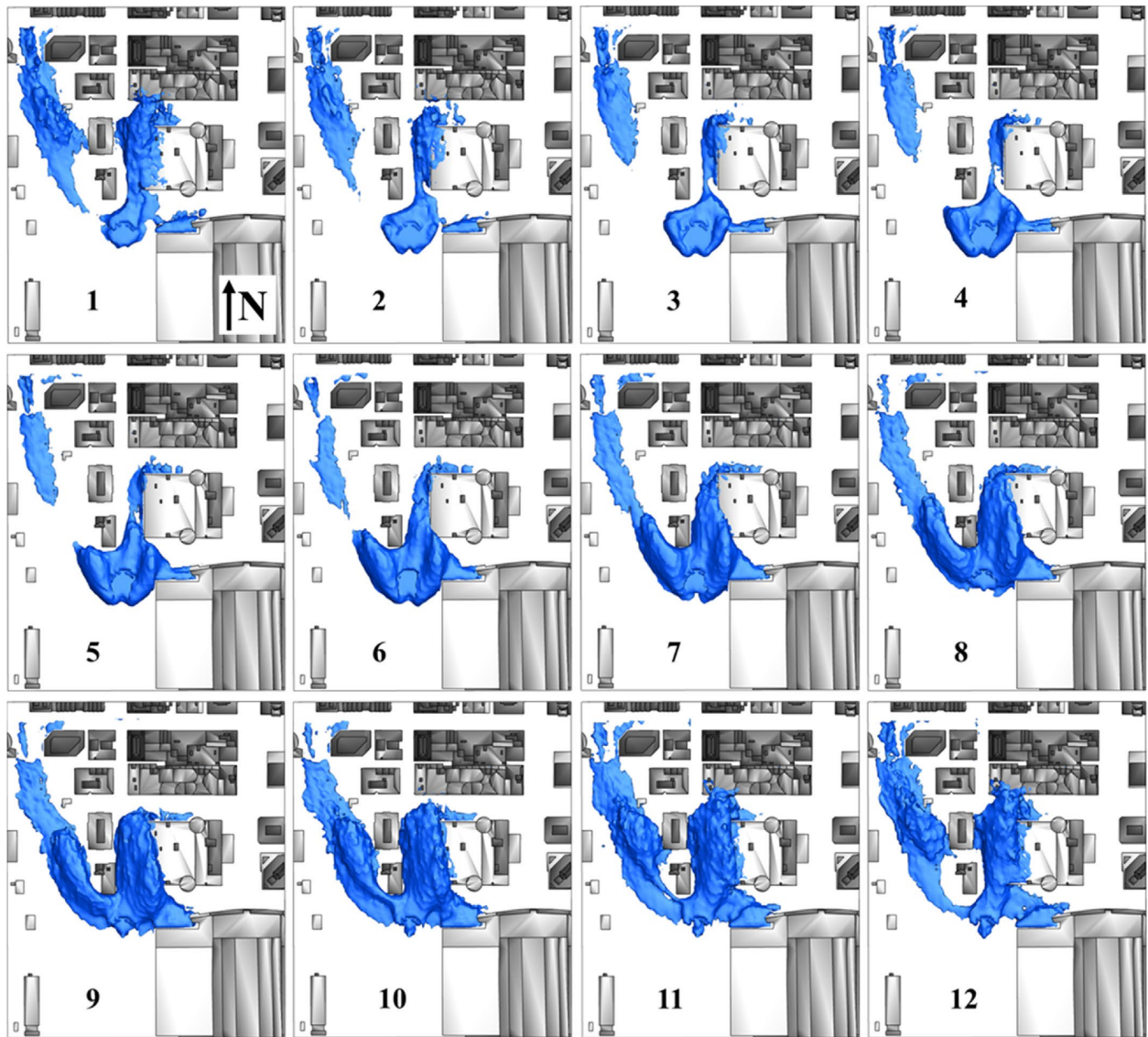
Figure. 2. Top view of isosurfaces at 8% concentration for each of the 12 phases illustrating how the scalar plume interacts with the buildings as it advects downstream. (from Homan et al. 2021)
