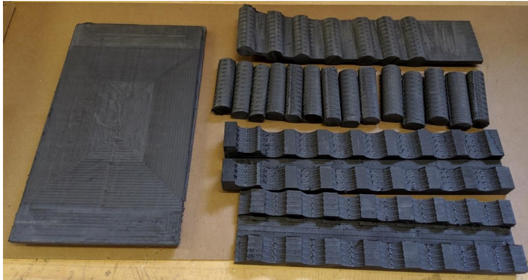
Figure 9 CNC-machined polyamide foam dunnage
