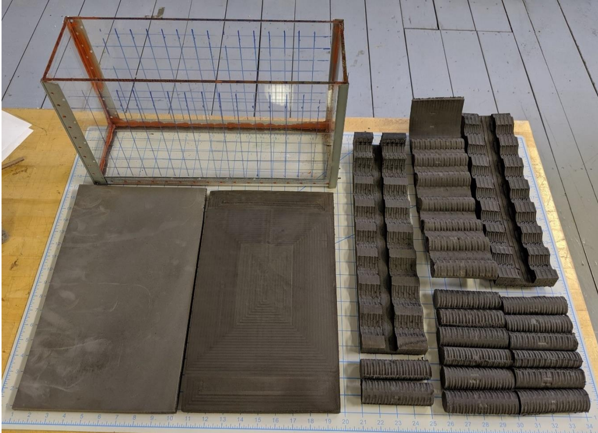
Figure 12 Polyamide dunnage post-test 3 (419 °F)
