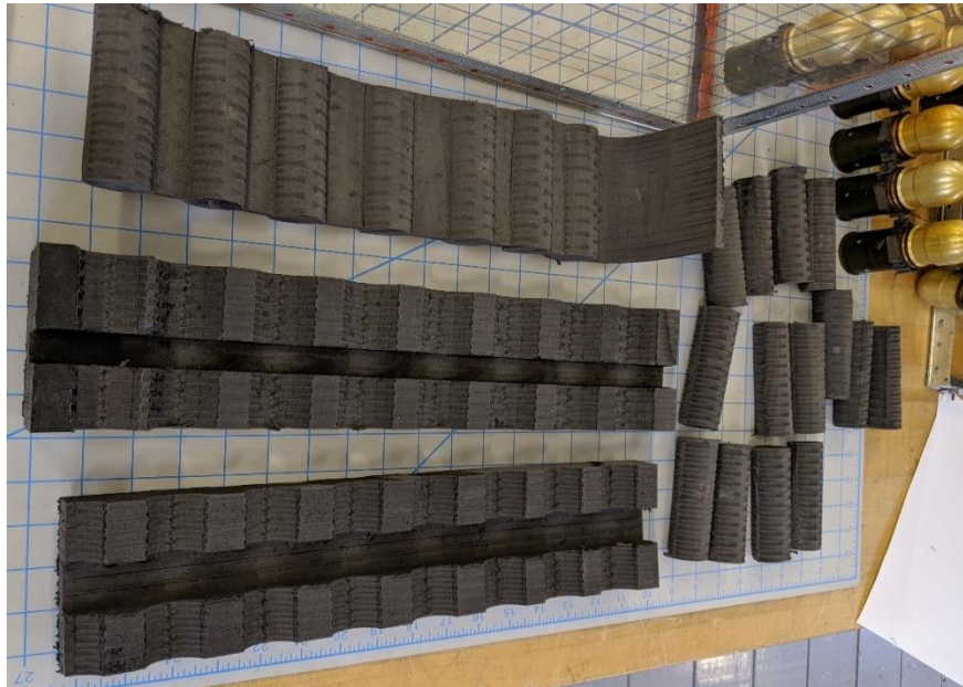
Figure 11 Polyamide dunnage post-test 2 (365 °F)
