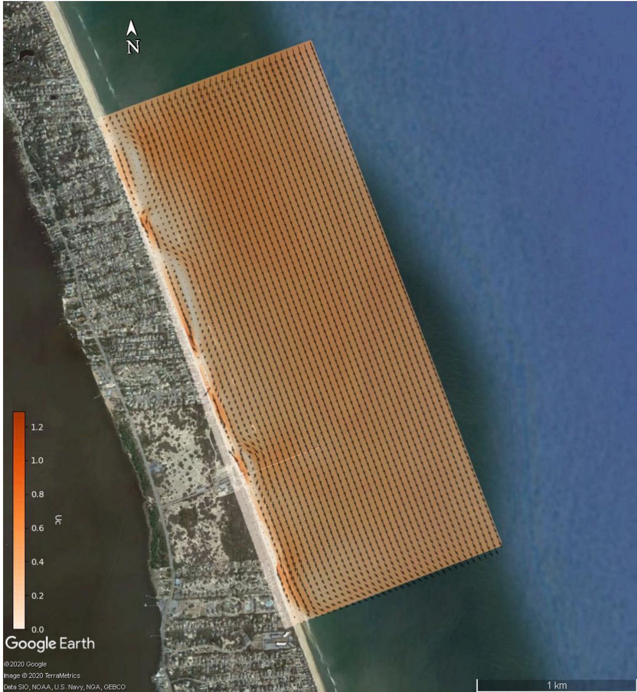
Figure 36. Depth-averaged current magnitude (color contours) and direction (black arrows) on 11 February 2015 0830 EST at the peak of the Northeaster storm.
