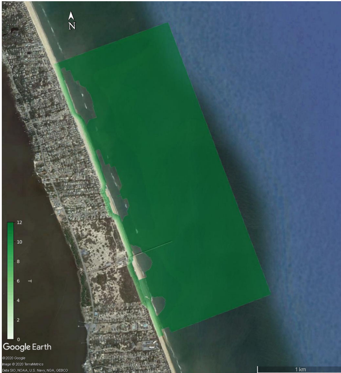
Figure 35. Peak wave period on 11 February 2015 0830 EST at the peak of the Northeaster storm used as input to UnMES. Regions near the shoreline where no model results are plotted indicate regions where the wave period exceeds the range with which the network was trained.
