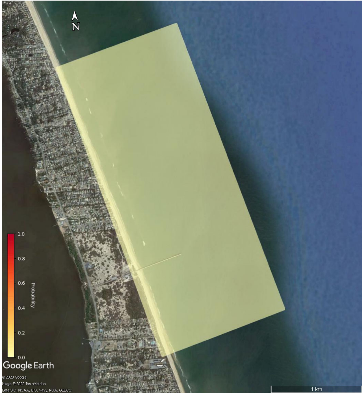
Figure 39. Estimated probability of surrogate 81-mm mortar remaining proud on the seafloor at the peak of the 11 February 2015 Northeaster.
