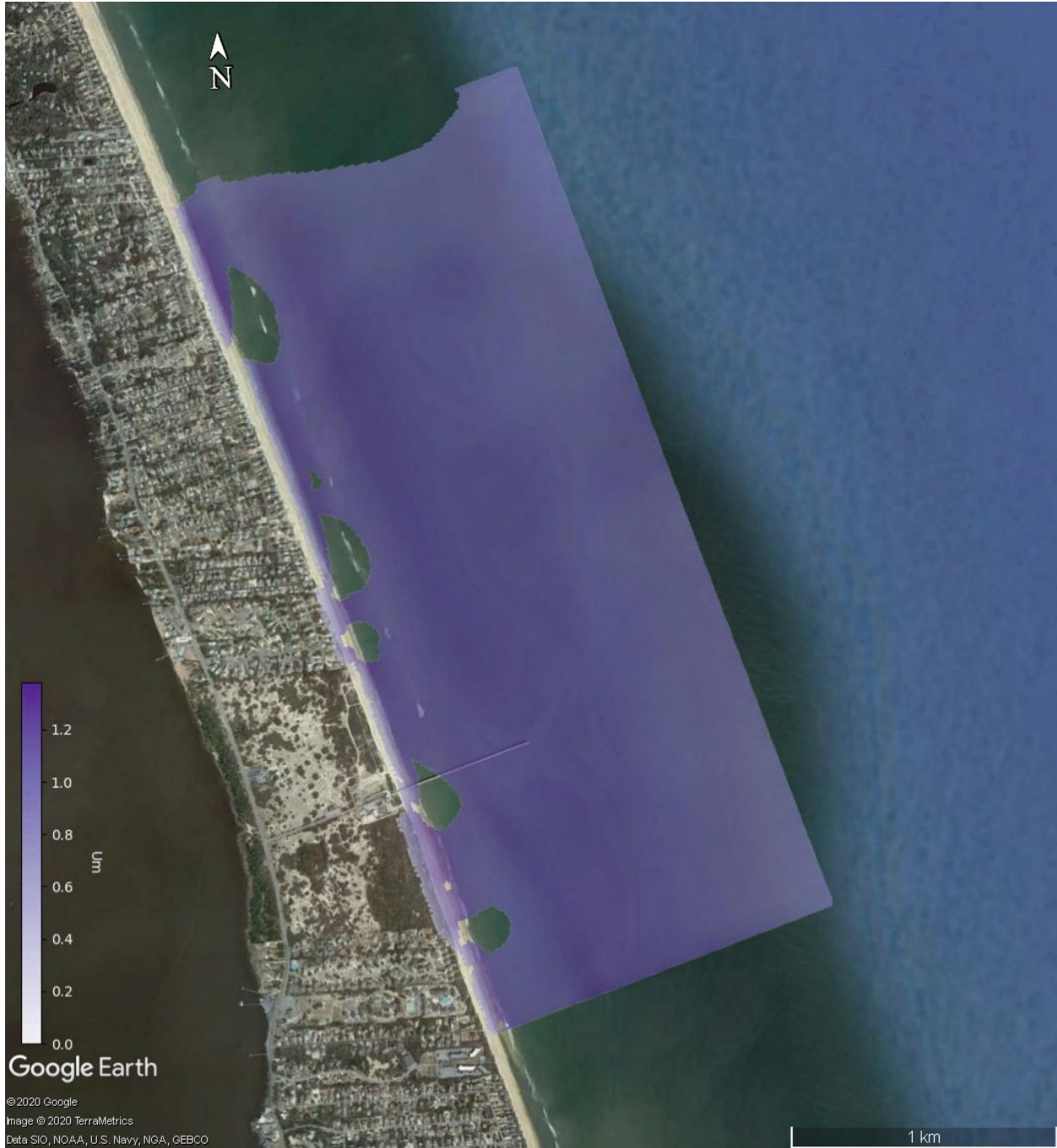
Figure 37. Near-bed combined wave and current magnitude on 11 February 2015 0830 EST at the peak of the Northeaster storm used as input to UnMES. Regions near the shoreline where no model results are plotted indicate regions where the variable value exceeds the range with which the network was trained.
