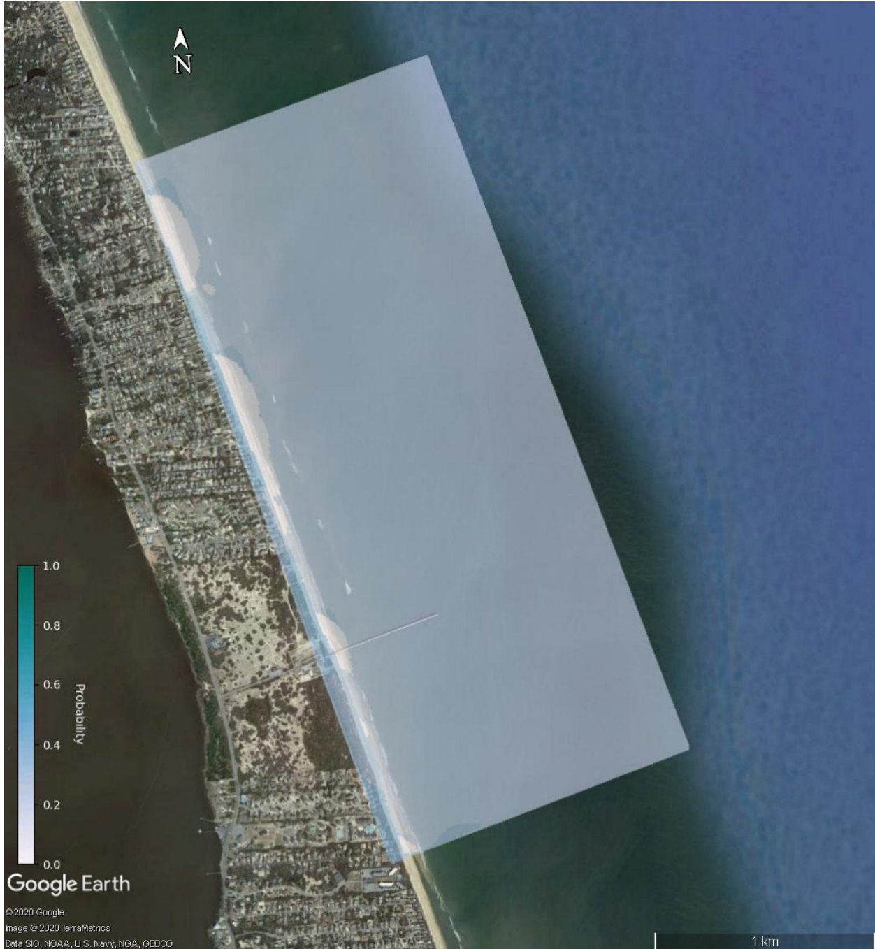
Figure 44. Estimated probability of surrogate 81-mm migrating towards the south ( 30^{\circ} - 135^{\circ} relative to shore normal) during the peak of the 11 February 2015 Northeaster.
