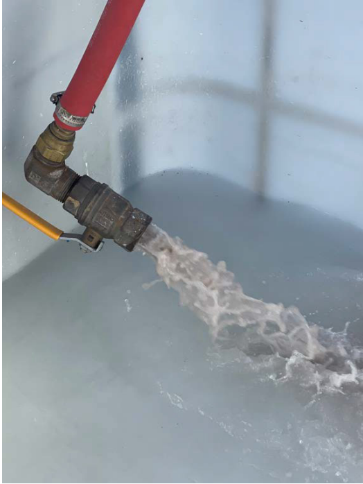
(a) Captured effluent during cutting exhibiting a darker color due to the abrasive.
