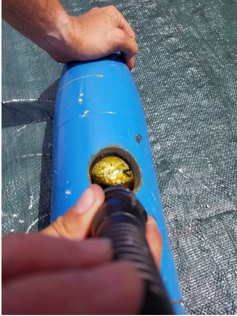
(a) Item #24 after cutting, plug removal, and incomplete washout.
