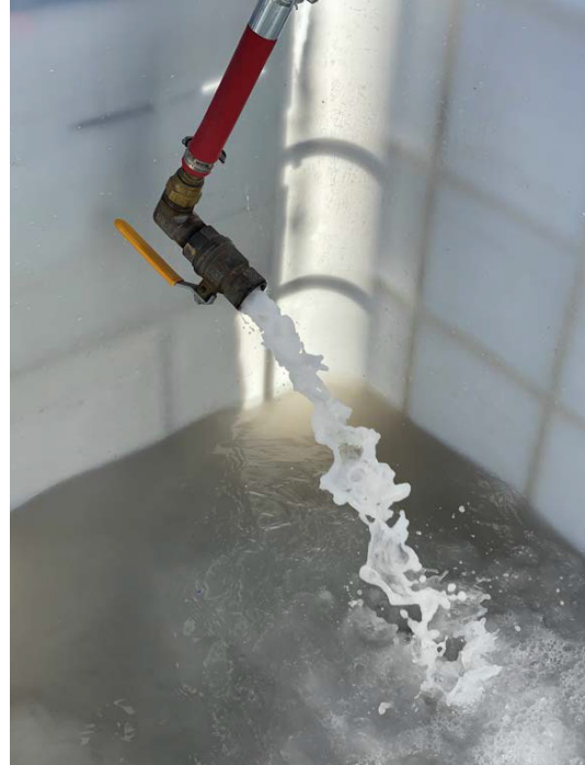
(b) Captured effluent during washout exhibiting a white color due to the cellulose.
