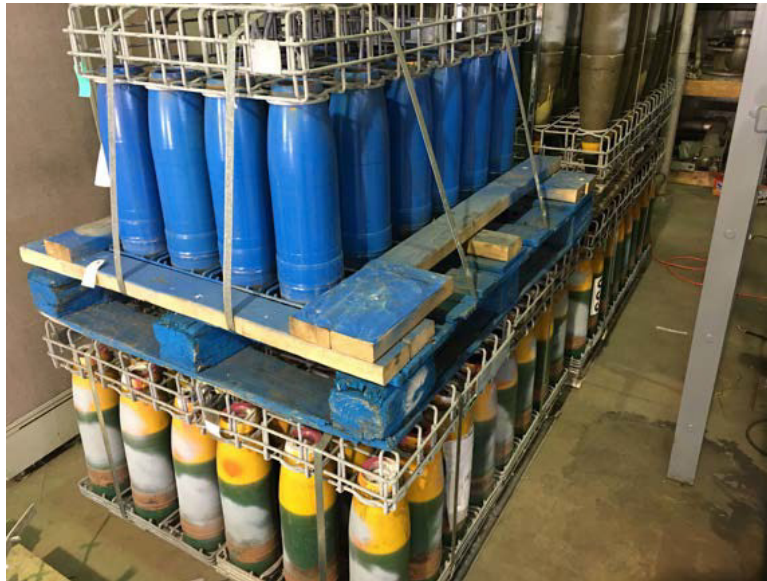
Figure 27. Demilitarized Navy 5-inch/38-caliber Projectiles that Were Used for Target Item Creation.
