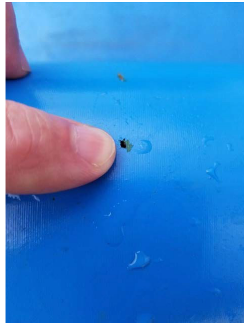
(d) Backside of item #21 showing a small hole pierced by the high-pressure waterjet during cutting.
