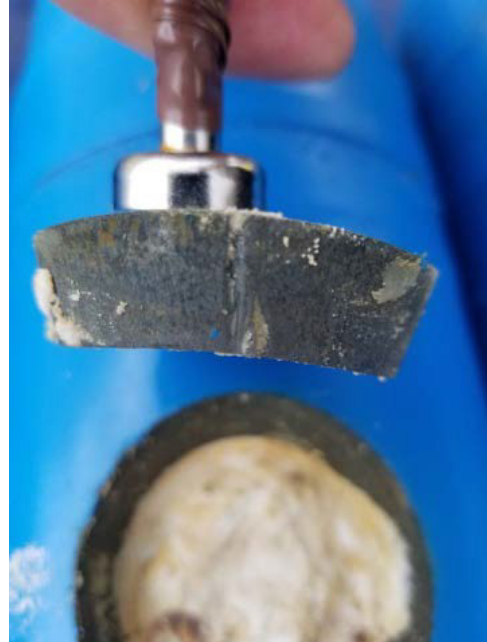
(b) This plug from item #37 is representative of others that contained a sliver of steel after cutting that prevented the plug from being removed with the magnet.
