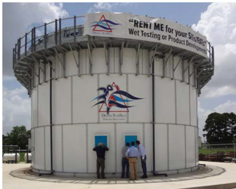
Figure 17. Delta SubSea's Tooling Test Tank that is 38.3 Feet in Diameter and 23.4 Feet Deep Holding 200, 567 Gallons of Water.
