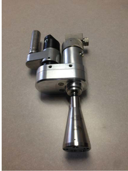
Figure 3. High-pressure Waterjet Cleaning Tool.
