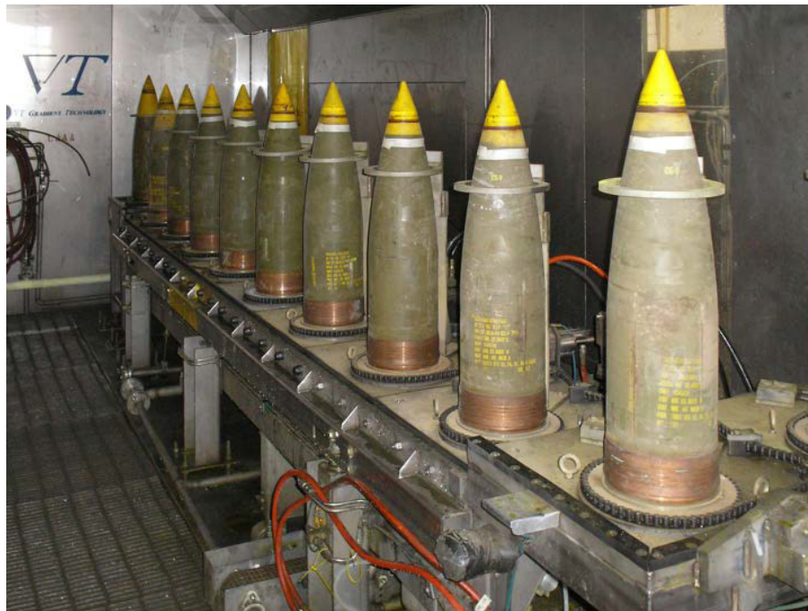
Figure 1. Automated AWJ Cutting and Washout System Processing 8-in/55-cal HC Rounds.
