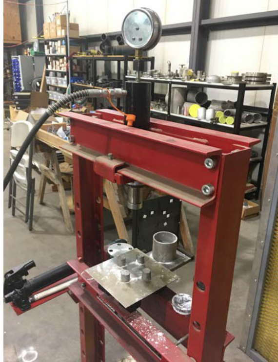
Figure 29. Hydraulic Press for Pressing the Inert Fill into the Target Items.
