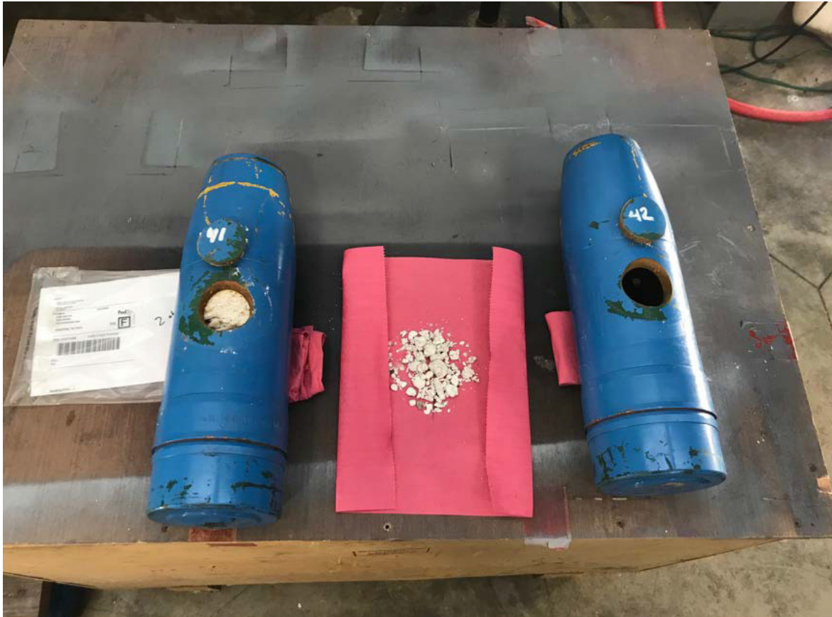
Figure 33. Inert Filled Projectiles after Cutting/Plug Removal and Washout.
