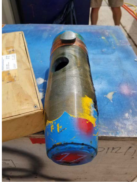
(b) Item #17 after concrete removal, cutting, plug removal, and washout.
