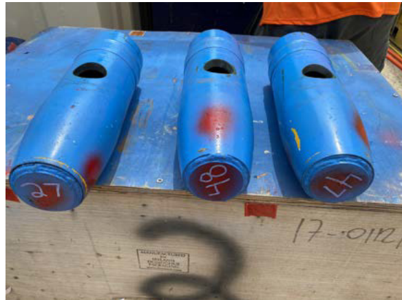
(d) Items #27, #47, and #48 after cutting, plug removal, and washout.
