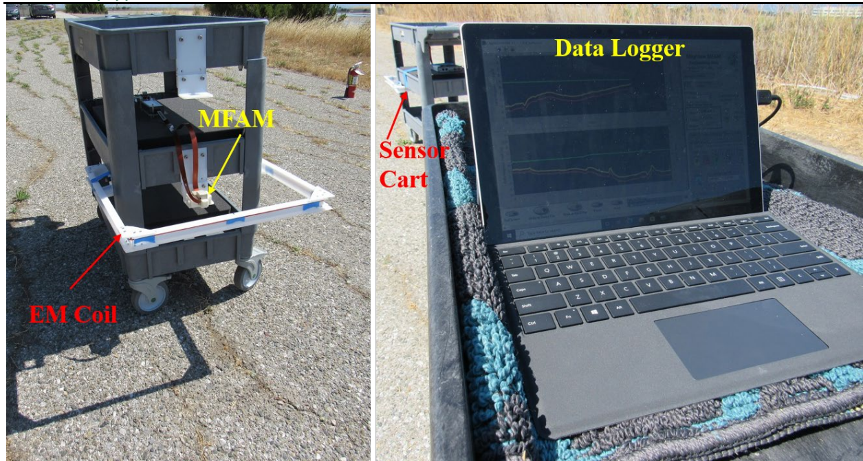
Figure 70 Advanced magnetometer setup. The system has an EM transmitter coil and the MFAM sensors. The data logger computer and the pulse generator is located in another cart 15 feet away.
