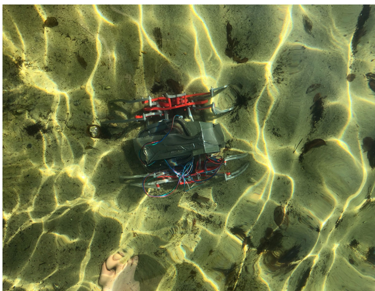
Fig. 21. Klann 2 robot walking at 1 meter depth in shallow inland lake
