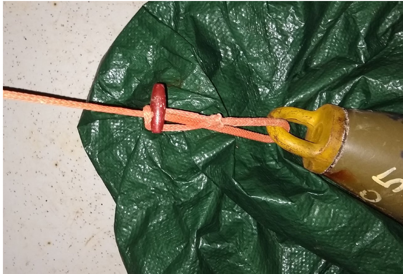
Figure 3. Wooden toggle button used to attach the tethers to the targets. A loop spliced into the end of the line was wrapped around the target and then "buttoned" onto the toggle.
