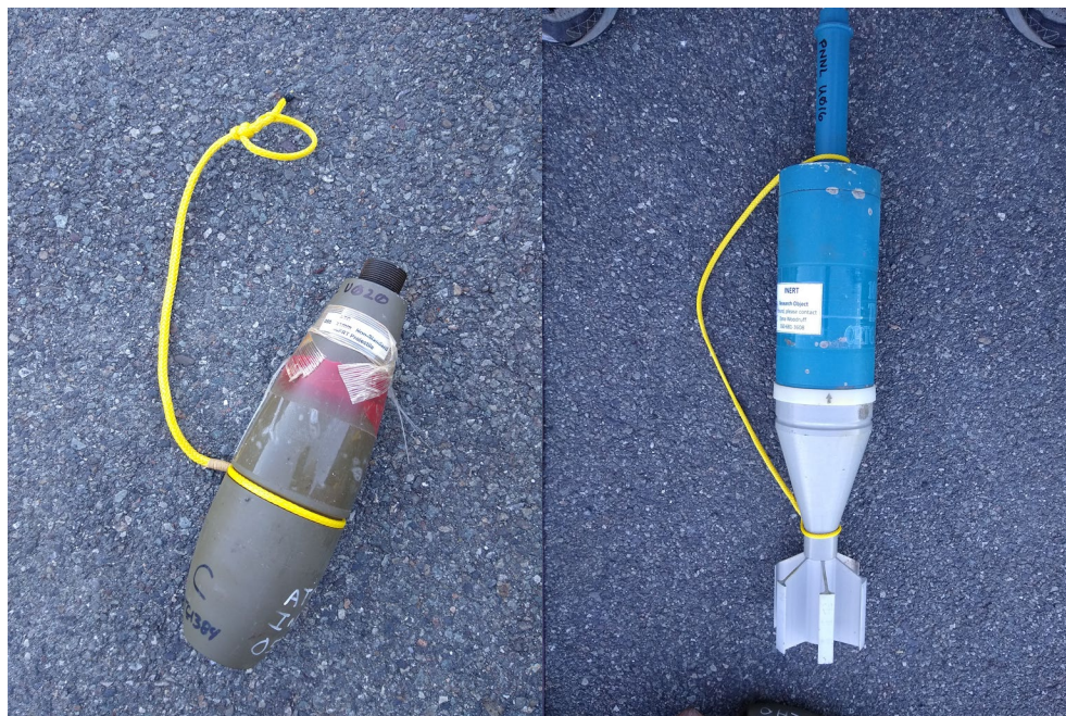
Figure 5. Examples of harnesses placed on a 81 mm mortar (left) and a 105 mm HEAT projectile (right).
