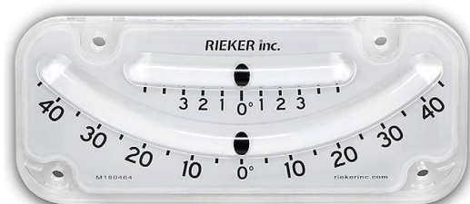
Figure 8. Inclinometer used to determine the pitch of the targets while on the bottom of Sequim Bay. Photo on the right shows the inclinometer being used on an 81 mm mortar during retrieval.
