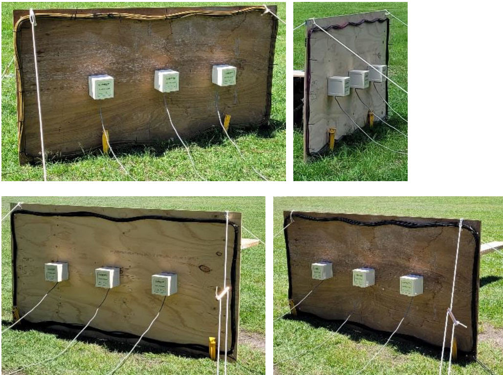
Figure 17. Proof-of-Concept testing of transmitter loop configurations. (top left) 16 turn, 4 mm 2 ; (top right) 8 turn, 25 mm 2 ; (bottom left) 12 turn, 6 mm 2 ; (bottom right) 10 turn, 10 mm 2 coils.
