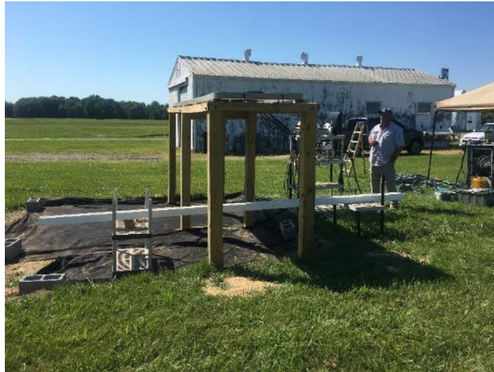
Figure 9. Setup for baseline signal measurements with the rail aligned fore-aft beneath the array.
