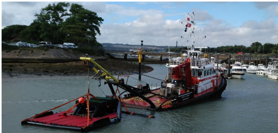
Figure 2. BTG/GapEOD/Boskalis SubTEM. For the Portsmouth project the SubTEM system was deployed on a sledge that was dragged over the sea-bottom
