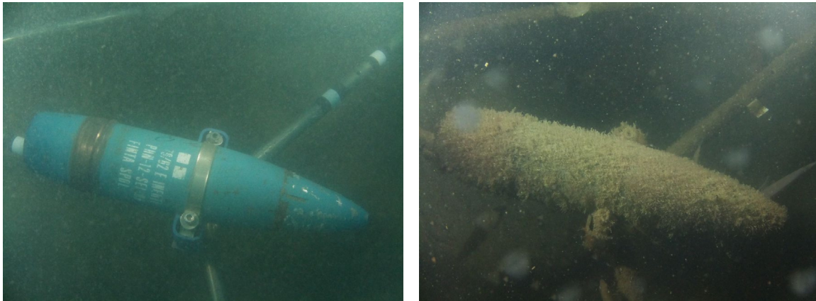
Figure 13. Target showing biofouling progression after 45 days.
